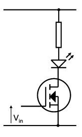
In this circuit an FET is connected to an LED, however it could be used to drive any load including higher power loads. When  $V_{in}$  is at zero volts the gate of the FET has no voltage on it and no current flows through the LED. When  $V_{in}$  is high the FET turns on and current flows through the FET from the drain to the source and the LED lights.
