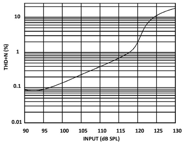
Figure 6. THD + N vs. Input Level
