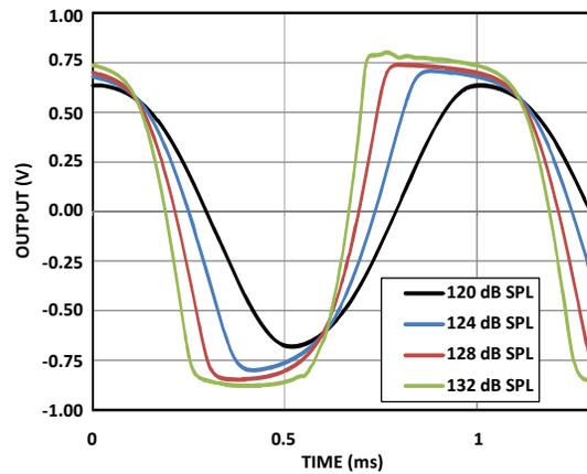
Figure 8 Clipping Characteristics
