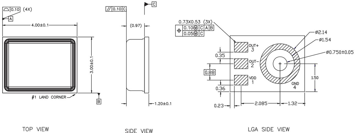
Figure 12. 4-Terminal Chip Array Small Outline No Lead Cavity
