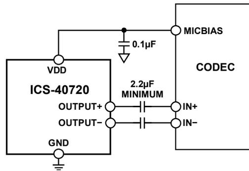
Figure 9. ICS-40720 Connected to a Differential-Input Codec
