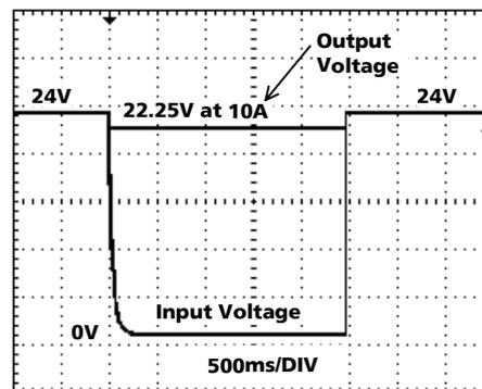
Fig. 7-3 Available output current in buffer mode
