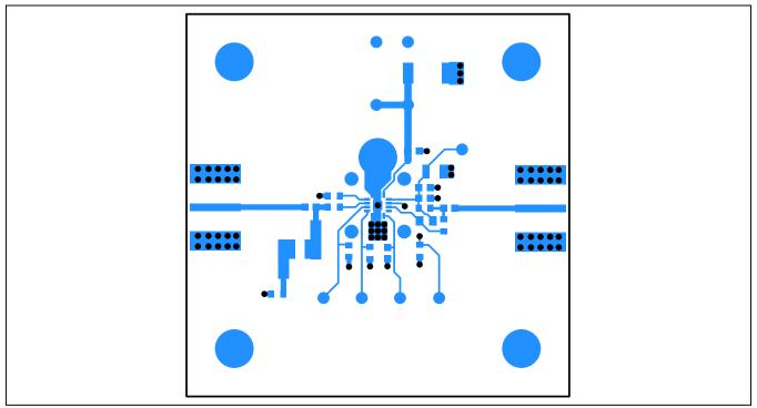
Figure 3. MAX2181 EV Kit PCB Layout—Top Copper
