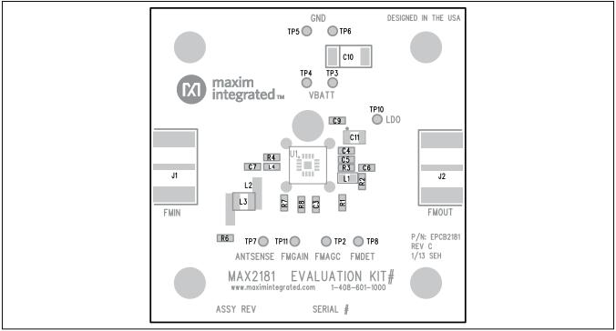
Figure 2. MAX2181 EV Kit Component Placement Guide—Top Silkscreen
