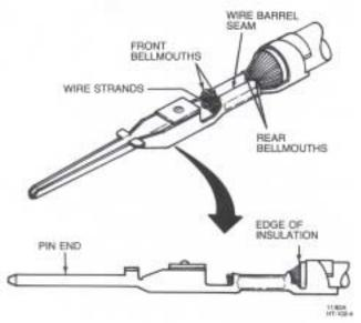
Figure 4. Correctly Crimped Terminal
