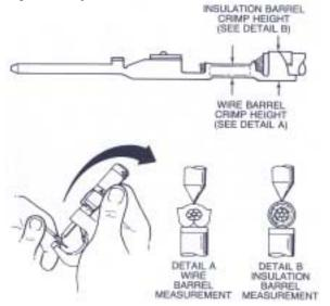
Figure 5. Measuring Crimp Height of Terminal
