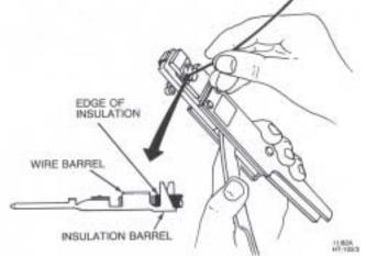
Figure 3. Crimping Terminal to Wire
