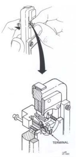
Figure 2. Positioning Terminal for Crimping
