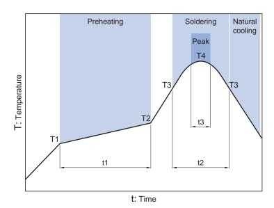
Preheating Soldering Peak Temp. Temp. Temp. Time Time Time T1 T2 T4 Т3 t3 150°C 180°C 60 to 120s 230°C 30 to 60s 250 to 260°C 10s max.
