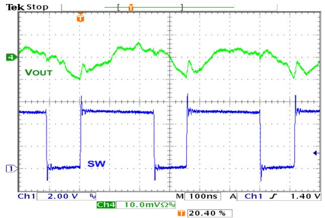
Figure 25. Output Ripple, 200 mA PWM Load
