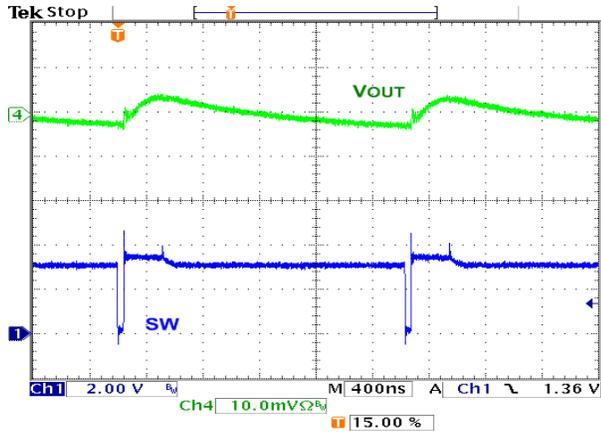
Figure 42. Output Ripple, 10 mA PFM Load
