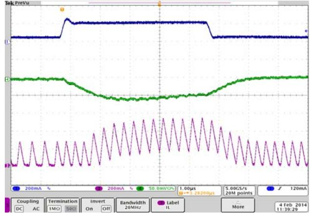
Figure 13. 50-200 mA Load Transient, 100 ns Step
