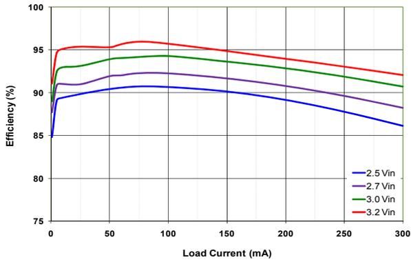
Figure 36. Efficiency vs. V<sub>IN</sub>
