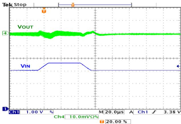
Figure 28. Line Transient, 5 mA Load, 10  $\mu\text{s}$  Step
