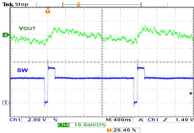
Figure 24. Output Ripple, 10 mA PFM Load
