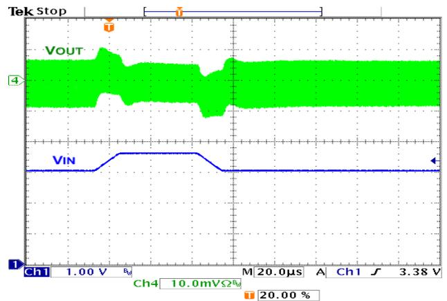
Figure 29. Line Transient, 200 mA Load, 10  $\mu\text{s}$  Step
