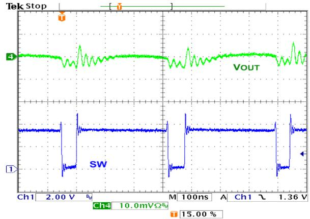
Figure 43. Output Ripple, 200 mA PWM Load
