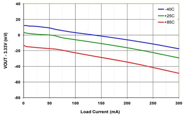
Figure 39. Load Regulation vs. Temperature, 3.0 V<sub>IN</sub>
