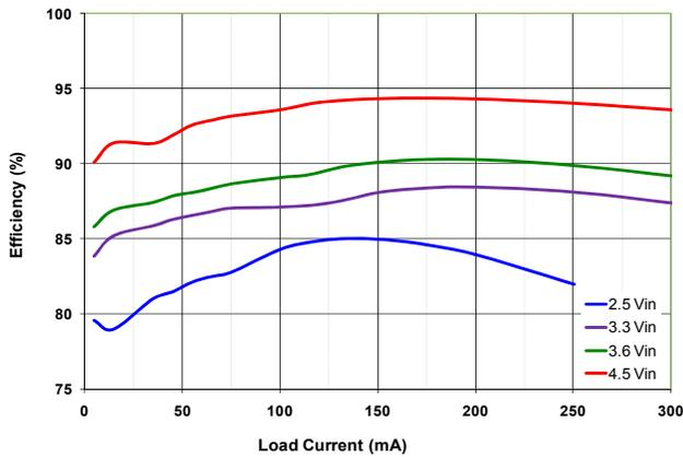
Figure 16. Efficiency vs. V<sub>IN</sub>
