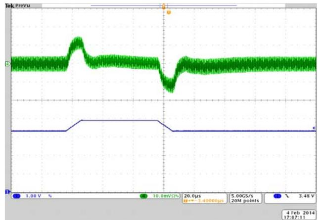
Figure 15. Line Transient, 200 mA Load, 10 µs Step
