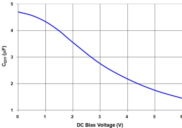
**Figure 50. C<sub>EFF</sub> for 4.7  $\mu$ F, 0603, X5R, 6.3 V (Murata GRM188R60J475K)**
