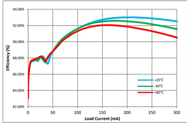
Figure 7. Efficiency vs. Temperature, 3.6 V<sub>IN</sub>
