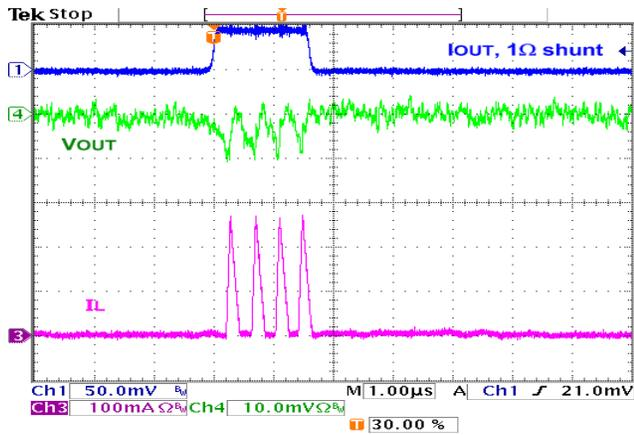
Figure 26. 0-50 mA Load Transient, 100 ns Step
