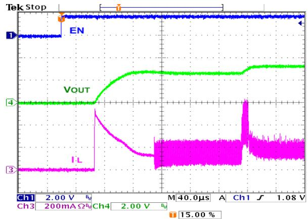
Figure 45. Startup, 22 Ω Load
