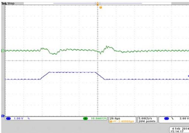
Figure 14. Line Transient, 5 mA Load, 10 µs Step
