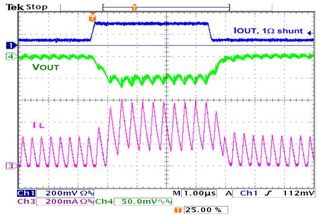
Figure 27. 50-200 mA Load Transient, 100 ns Step
