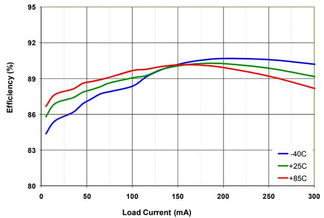
Figure 17. Efficiency vs. Temperature, 3.6 V<sub>IN</sub>
