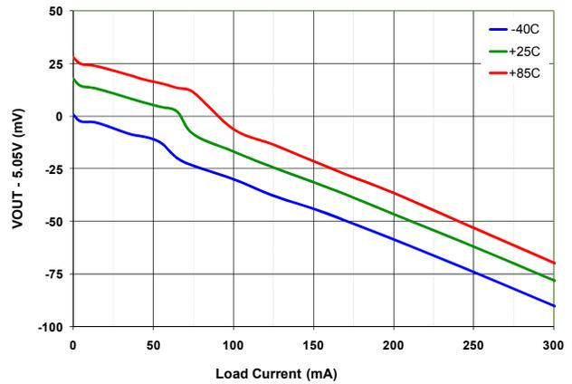
Figure 19. Load Regulation vs. Temperature, 3.6 V<sub>IN</sub>
