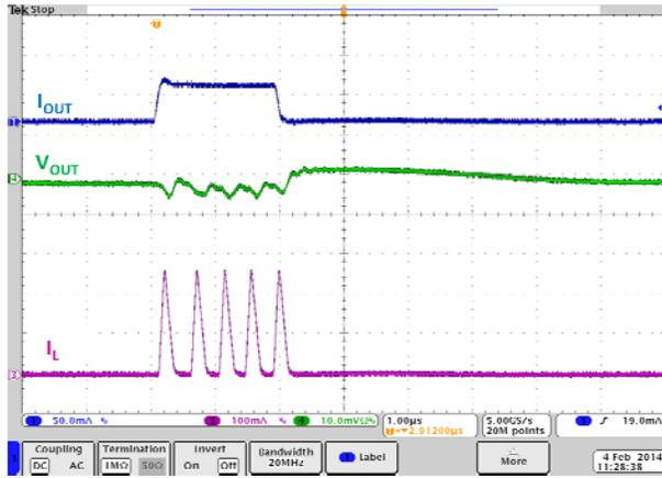
Figure 12. 0-50 mA Load Transient, 100 ns Step
