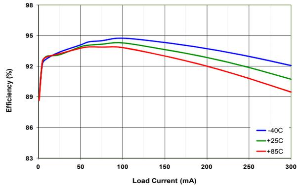
Figure 37. Efficiency vs. Temperature, 3.0 V<sub>IN</sub>
