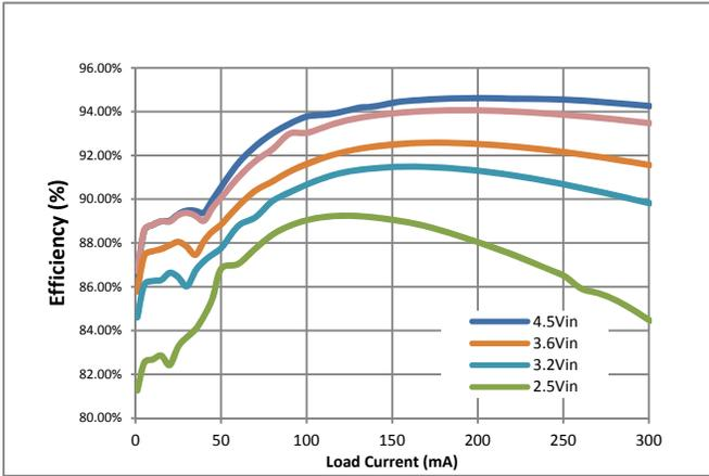
Figure 6. Efficiency vs. V<sub>IN</sub>
