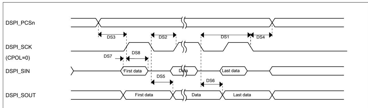
**Figure 34. DSPI classic SPI timing — master mode**
