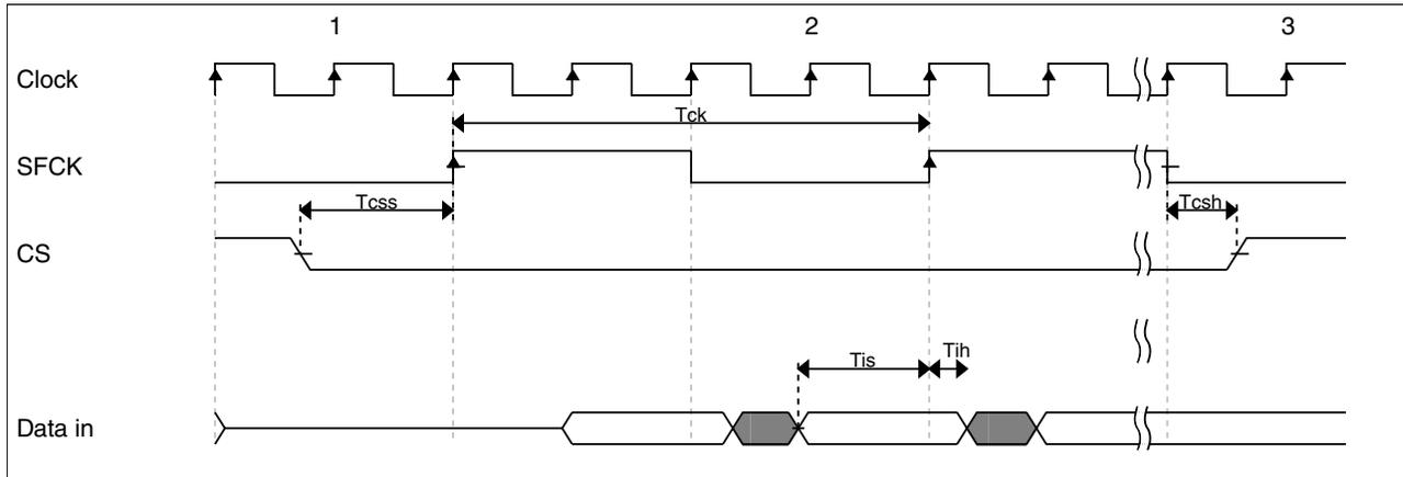
**Figure 16. QuadSPI input timing (DDR mode) diagram**
