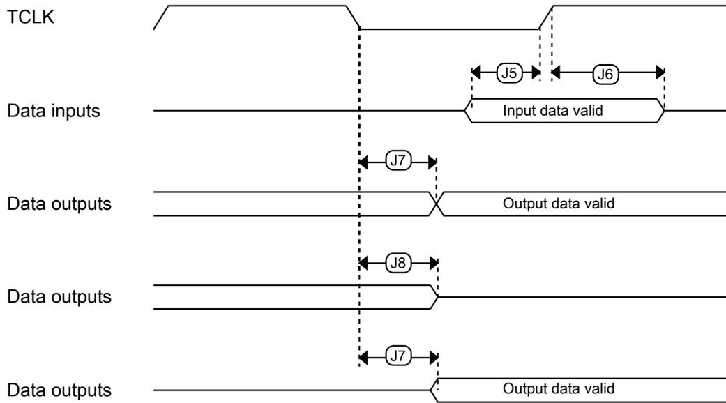
Figure 11. Boundary scan (JTAG) timing
