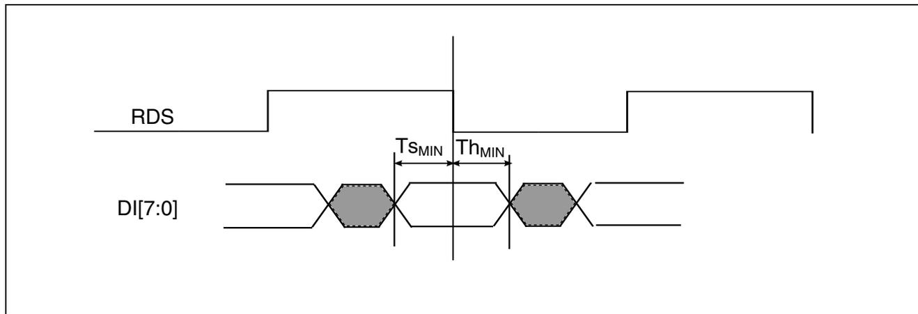
**Figure 18. QuadSPI input timing (Hyperflash mode) diagram**
