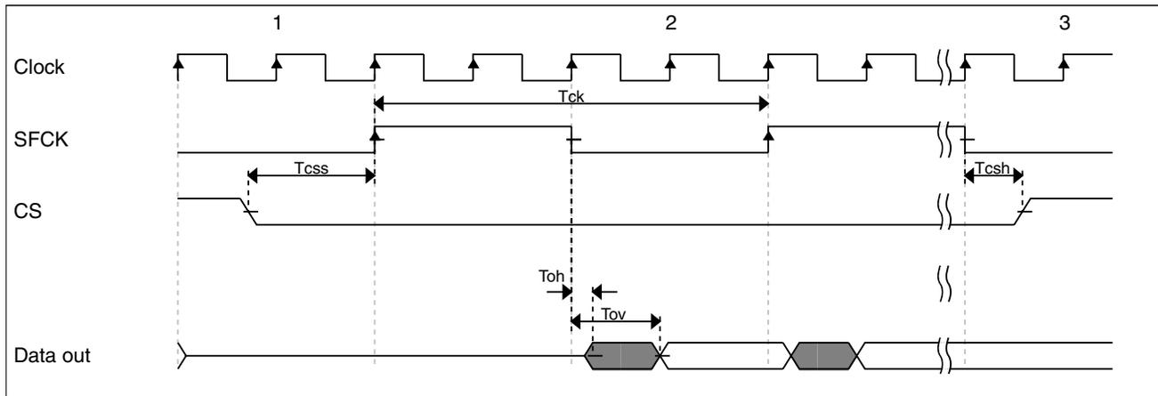
**Figure 15. QuadSPI output timing (SDR mode) diagram**
