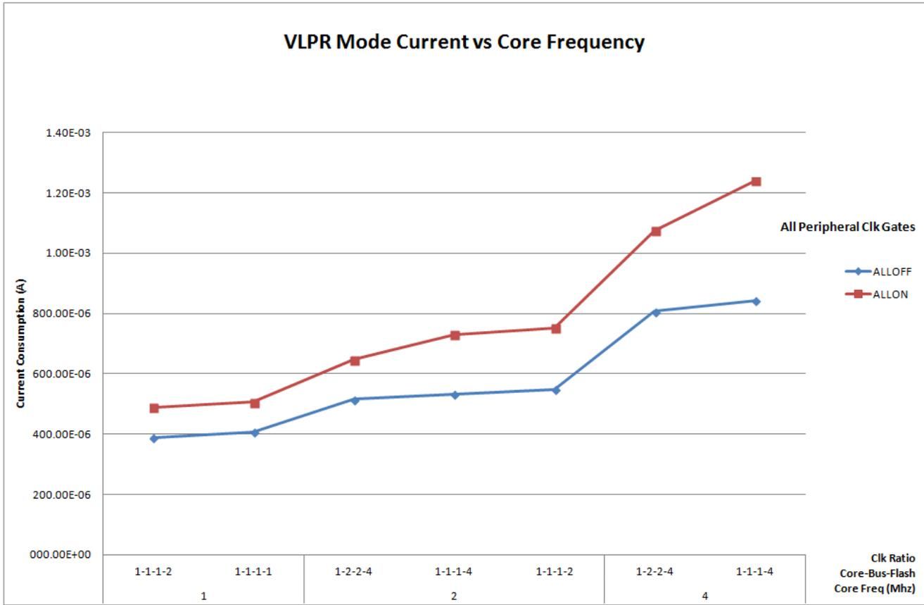
Figure 7. VLPR mode supply current vs. core frequency
