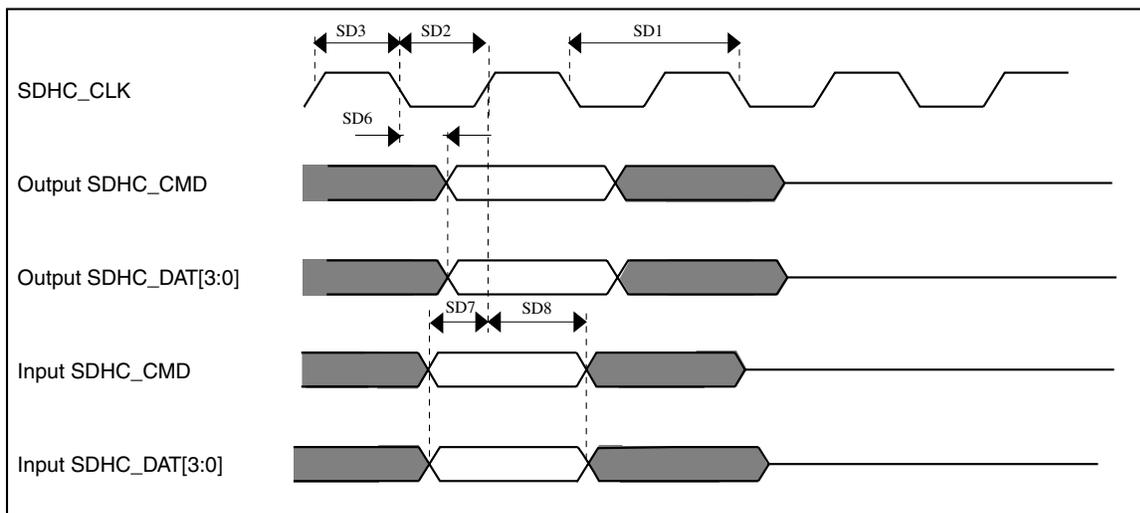
**Figure 38. SDHC timing**
