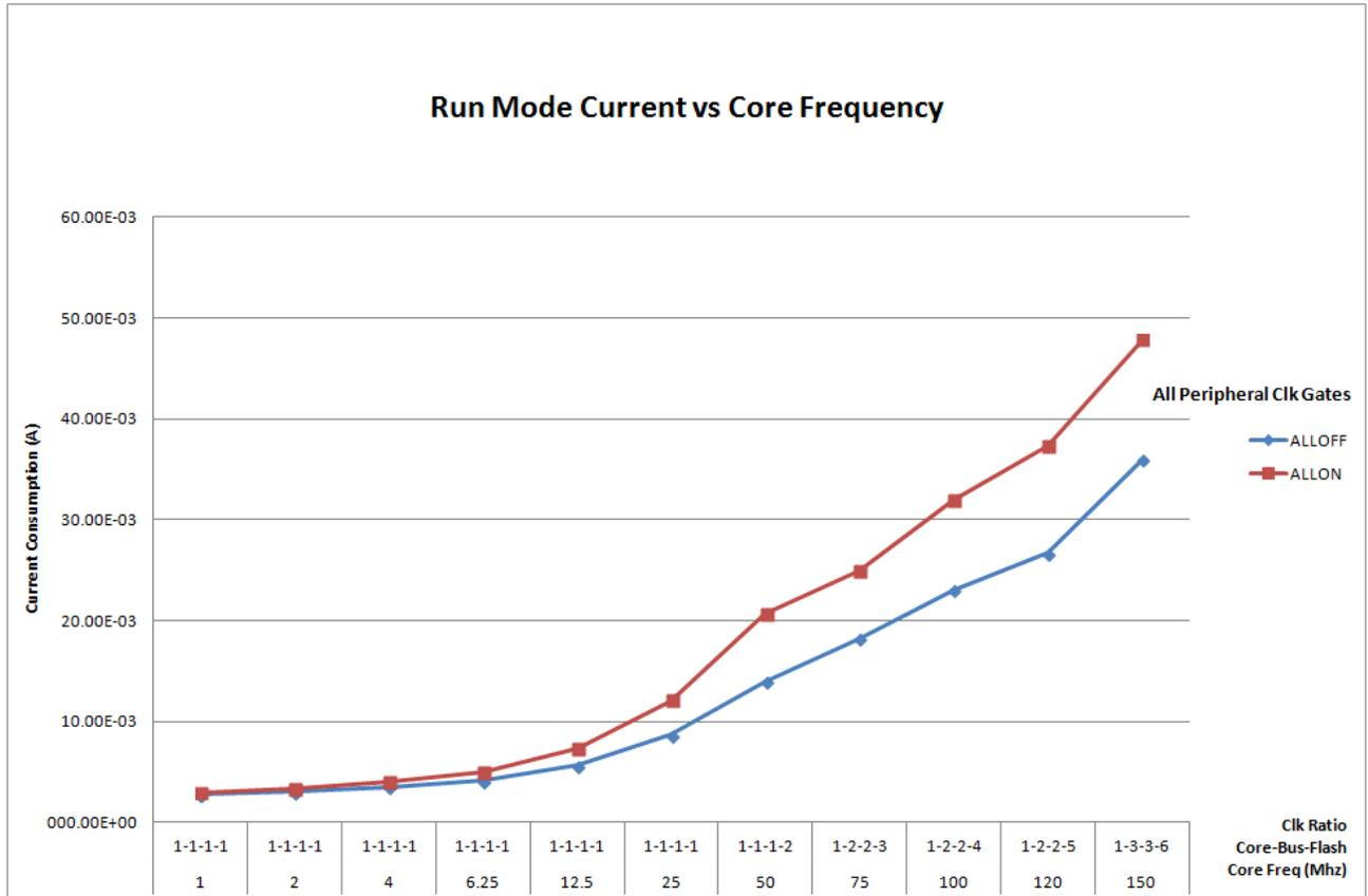
**Figure 6. Run mode supply current vs. core frequency**
