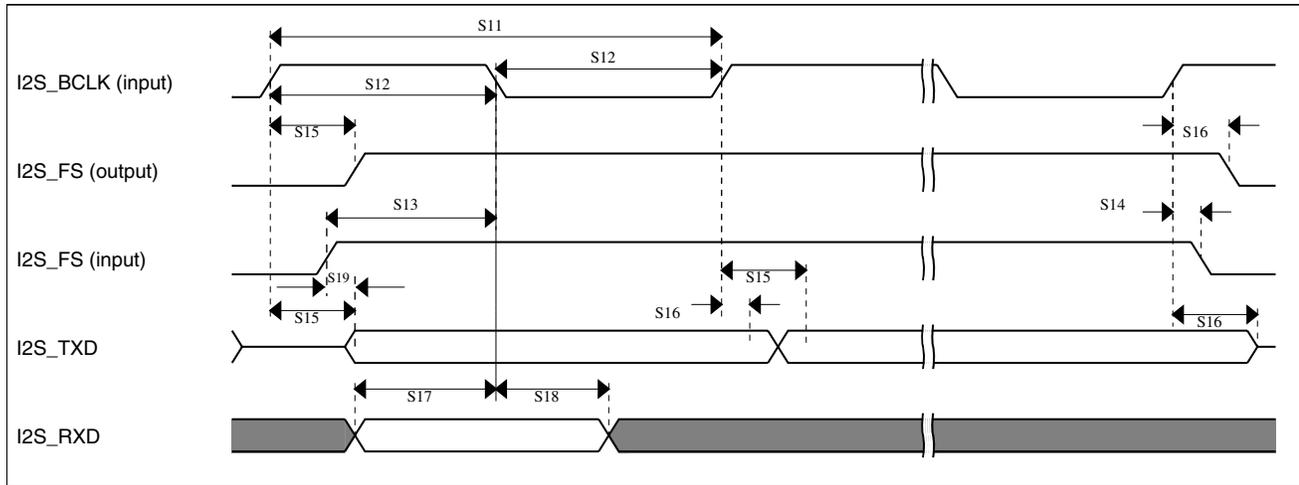
Figure 40. I<sup>2</sup>S timing — slave modes
