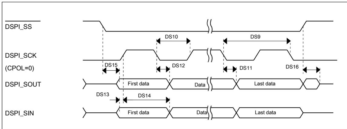
**Figure 35. DSPI classic SPI timing — slave mode**
