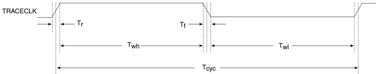
**Figure 8. TRACE\_CLKOUT specifications**
