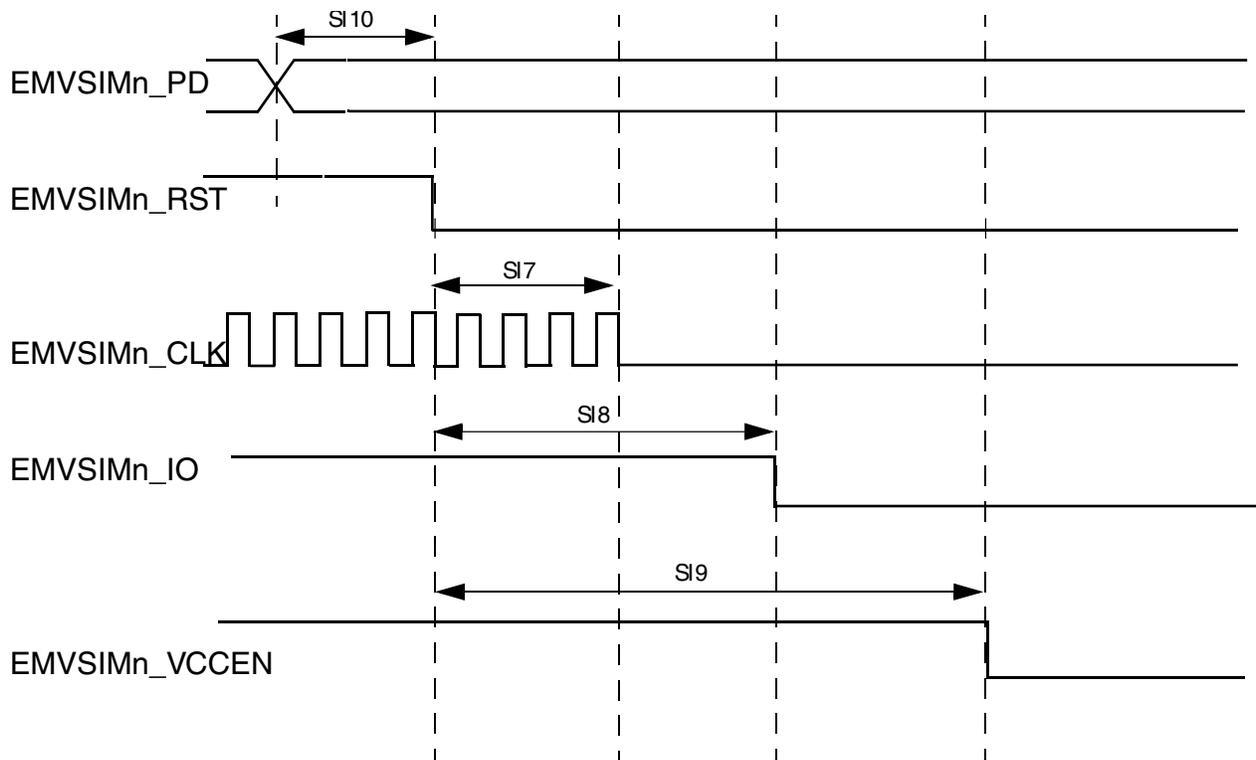
**Figure 33. Smart Card Interface Power Down AC Timing**
