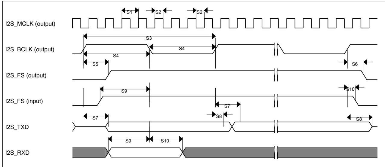
**Figure 39. I<sup>2</sup>S timing — master mode**
