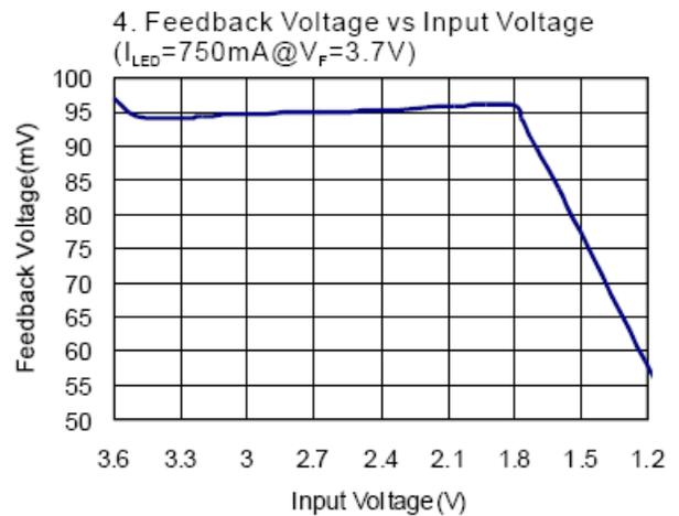
**Typical Performance Characteristics** (cont.) @ $T_A = +25^\circ\text{C}$ ,  $L = 2.2\mu\text{F}$ ,  $C_{IN} = 10\mu\text{F}$ ,  $C_O = 10\mu\text{F}$ , unless otherwise specified.)
