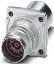
Panel feed-through, straight, SPEEDCON locking, M17, Number of positions: 8, Type of contact: Socket, Crimp connection, Flat gasket, 4x Ø3.2, shielded: yes, Flange dimensions: 25.75 mm x 25.75 mm, Cable diameter: 9 mm...11 mm
