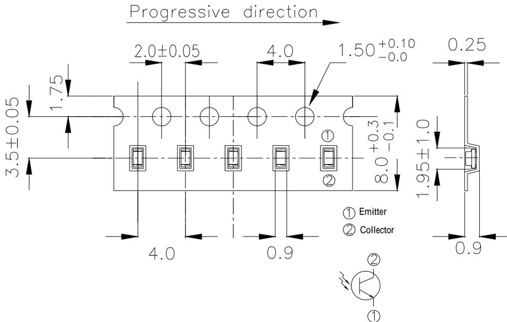
**Note:** The tolerances unless mentioned are  $\pm 0.1$ mm, Unit: mm
