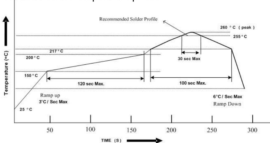
3.2 Reflow soldering should not be done more than two times.
