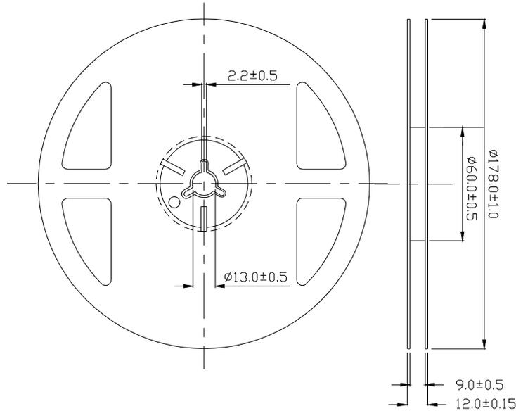
**Note:** The tolerances unless mentioned are  $\pm 0.1$ mm, Unit: mm
