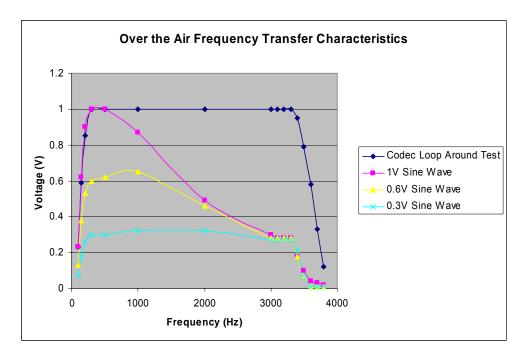
As can be seen, the frequency response can only be considered to be flat when the input voltage level is less than a 0.3V peak to peak sine wave.
