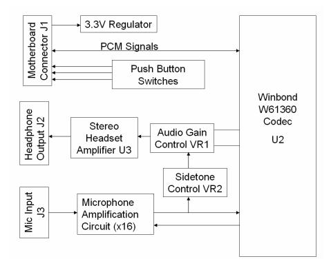
The codec board is powered by an on-board 3.3V regulator to reduce noise to a minimum. The PCM control signals for the codec go directly to the *Bluetooth* module on the motherboard via the 10-way connector, as do the 3 push button switches. This allows the switches to be used with an external program that implements the upper portion of headset or Handsfree profile.
