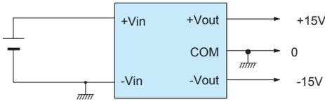
■ When a floating mechanism is required for the output circuit
