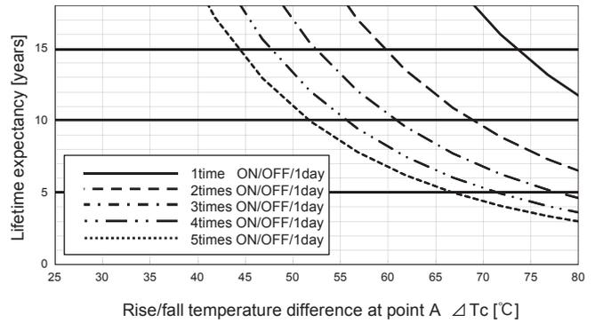
Fig.10.4 Lifetime expectancy against rise/fall temperature difference (MG6)
