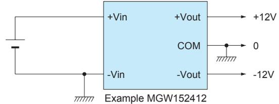
\* The unit can be used as a 24V type single output power supply as follows.
