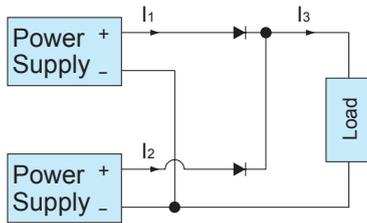
Fig.4.2 Redundancy Operation
