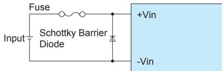
Fig3.2 Reverse Input Voltage Protection
