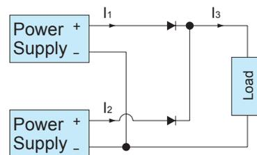
Fig.4.2 Redundancy operation
