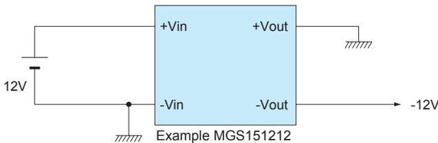
■ To provide a negative voltage to -Vin by using +Vin side of the converter as GND potential (0V)
