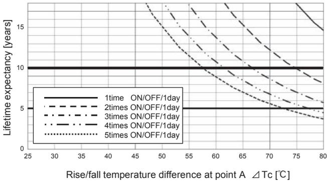
Fig.10.1 Lifetime expectancy against rise/fall temperature difference (MG1R5)
