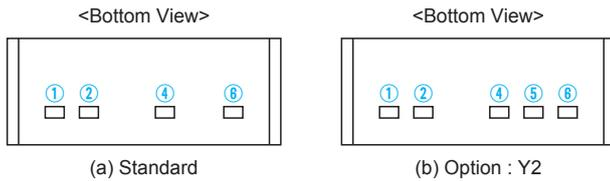
Fig.1.1 Pin Configuration(MG1R5/MG3 Single Output)
