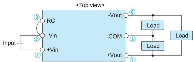
Fig.1.2 Pin Configuration (MG30)
