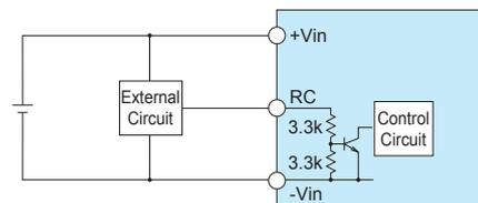
Fig.2.1 Internal Circuits of Remote ON/OFF
