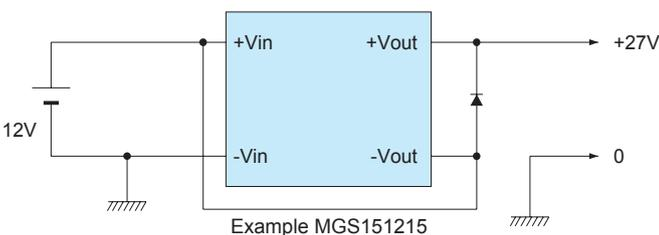
\* Output current should be the same as the rated output current of the converter.
