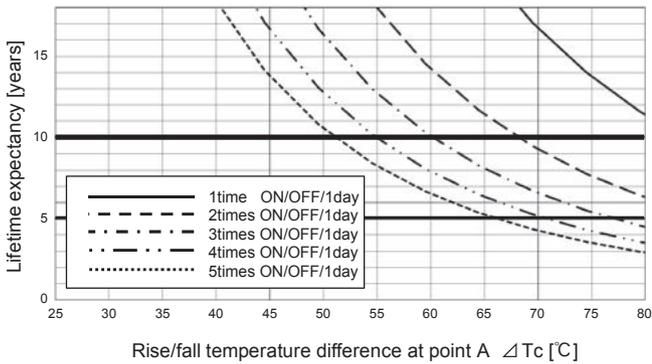
Fig.10.2 Lifetime expectancy against rise/fall temperature difference (MG3)
