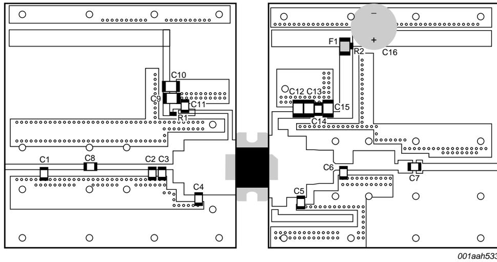
The striplines are on a double copper-clad Taconic RF35 Printed-Circuit Board (PCB) with  $\epsilon_r = 3.5$  and thickness = 0.76 mm. See [Table 8](#) for list of components.
