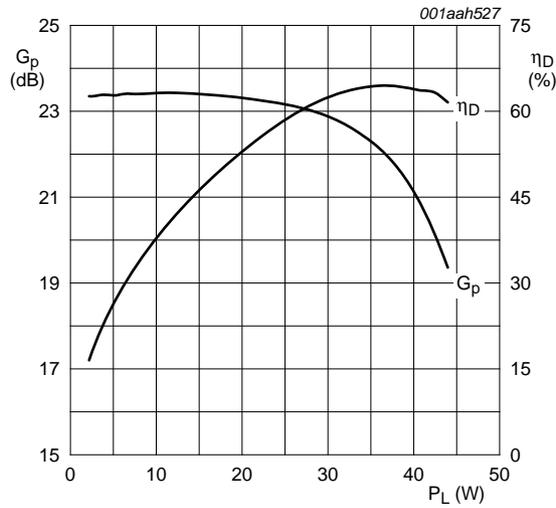
$V_{DS} = 28$  V;  $I_{Dq} = 350$  mA;  $f = 960$  MHz.
