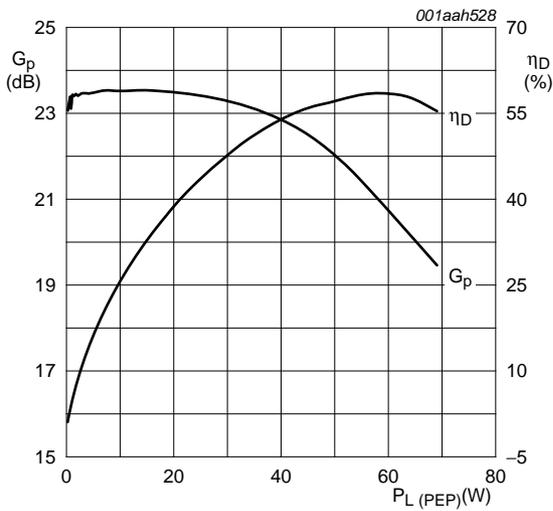
$V_{DS} = 28$  V;  $I_{Dq} = 350$  mA;  $f_1 = 960$  MHz;
