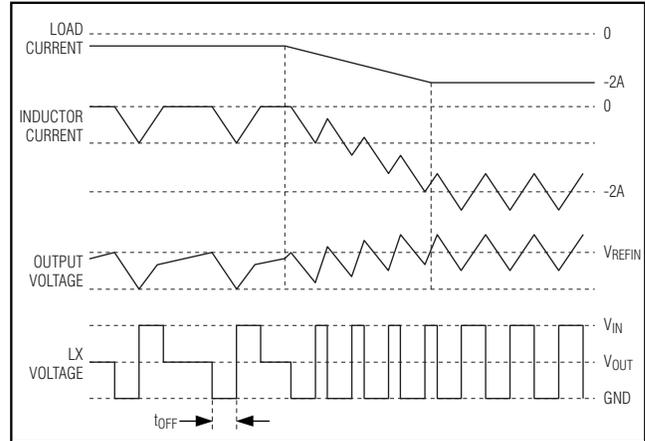
Figure 4. Sink-Mode Waveforms
