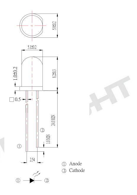
Note: Tolerances unless dimensions ±0.25mm
