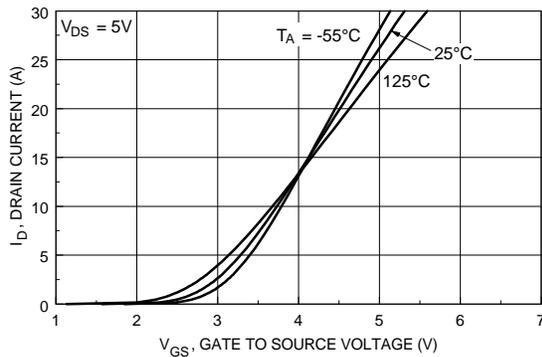
Figure 5. Transfer Characteristics.
