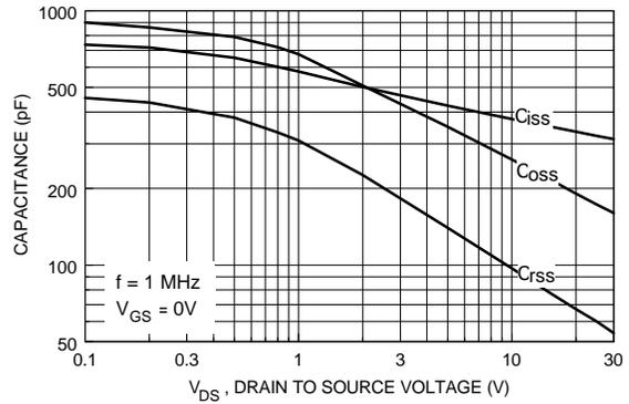
Figure 8. Capacitance Characteristics.
