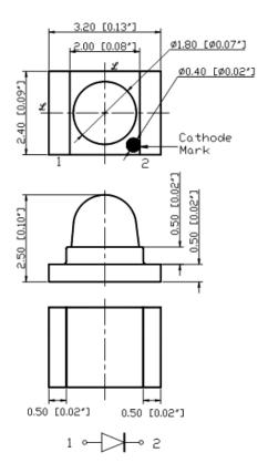
Units: mm / tolerance = +/-0.1mm
