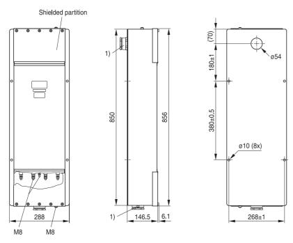
$<sup>^{1)}</sup>$  Cable glands PG 42\* with indented sealing ring, for cable diameters [mm]: 29  $\dots$  31 / 32  $\dots$  34 / 35  $\dots$  37 / 38  $\dots$  40
