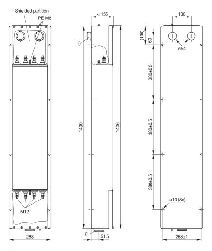
$<sup>^{1)}</sup>$  Cable glands PG 42\* with indented sealing ring, for cable diameters [mm]: 29 ... 31 / 32 ... 34 / 35 ... 37 / 38 ... 40  $^{2)}$  Cable glands PG 48\* with indented sealing ring, for cable diameters [mm]: 38 ... 41 / 42 ... 44 / 45 ... 47 / 48 ... 51
