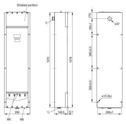
$<sup>^{1)}</sup>$  Cable glands PG 29\* with indented sealing ring, for cable diameters [mm]: 17  $\dots$  19 / 20  $\dots$  22 / 23  $\dots$  25 / 26  $\dots$  28
