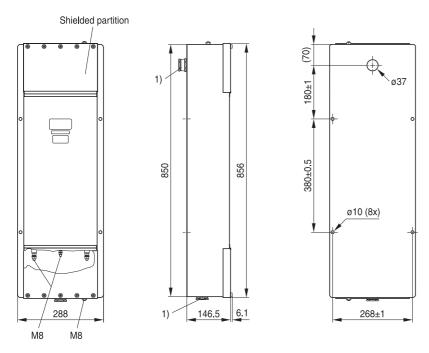
$<sup>^{1)}</sup>$  Cable glands PG 29\* with indented sealing ring, for cable diameters [mm]: 17  $\dots$  19 / 20  $\dots$  22 / 23  $\dots$  25 / 26  $\dots$  28
