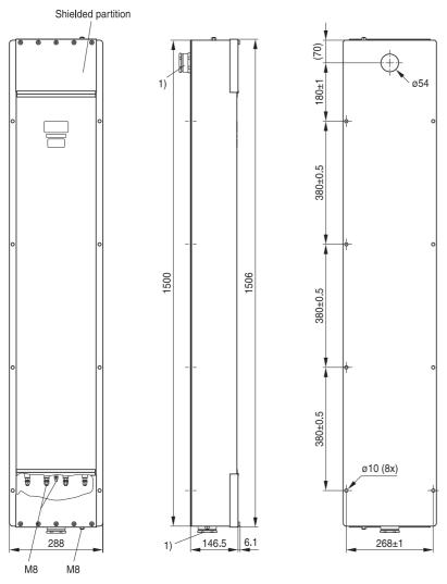
$<sup>^{1)}</sup>$  Cable glands PG 42\* with indented sealing ring, for cable diameters [mm]: 29 ... 31 / 32 ... 34 / 35 ... 37 / 38 ... 40
