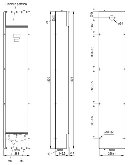
$<sup>^{1)}</sup>$  Cable glands PG 42\* with indented sealing ring, for cable diameters [mm]: 29  $\dots$  31 / 32  $\dots$  34 / 35  $\dots$  37 / 38  $\dots$  40
