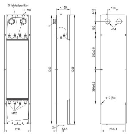
$<sup>^{1)}</sup>$  Cable glands PG 42\* with indented sealing ring, for cable diameters [mm]: 29 ... 31 / 32 ... 34 / 35 ... 37 / 38 ... 40  $^{2)}$  Cable glands PG 48\* with indented sealing ring,
