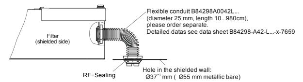
Note: The bending radius of the flexible conduit depends on the used type of cable
