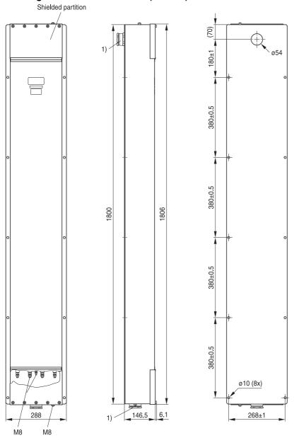
$<sup>^{1)}</sup>$  Cable glands PG 42\* with indented sealing ring, for cable diameters [mm]: 29  $\dots$  31 / 32  $\dots$  34 / 35  $\dots$  37 / 38  $\dots$  40
