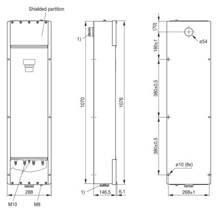
$<sup>^{1)}</sup>$  Cable glands PG 42\* with indented sealing ring, for cable diameters [mm]: 29  $\dots$  31 / 32  $\dots$  34 / 35  $\dots$  37 / 38  $\dots$  40
