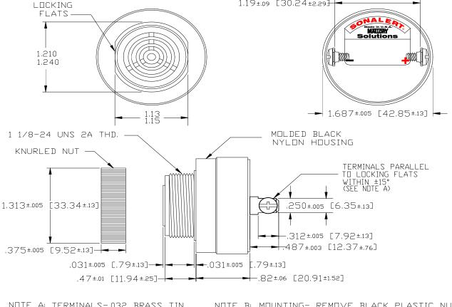
NOTE A: TERMINALS-.032 BRASS TIN PLATED, TAPPED FOR #6-32 TWO #6-32 NICKEL SCREW. PLATED BRASS SCREWS INCLUDED. WILL ACCEPT 1/4" QUICK CONNECT.
