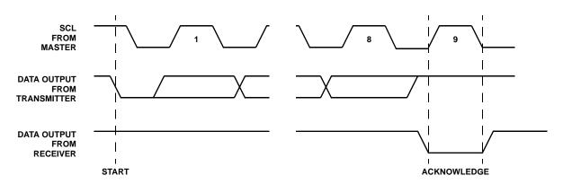
FIGURE 4. ACKNOWLEDGE RESPONSE FROM RECEIVE
