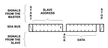
FIGURE 9. CURRENT ADDRESS READ SEQUENCE
