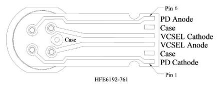
LC TOSA All dimensions in mm 0.13 MAX RELIEF BOTH SIDES Ø5.08+0.02 5.94-0.05 0.76 MAX -Ø6.6+0.02  $0.66\pm0.03$ PIN 1 IDENTIFIER  $6.28 \pm 0.02$ 14.09±0.17  $-02.92\pm0.02$ 4.04<sup>+0.05</sup> -0.02  $1.27\pm0.03$ OPTICAL PLANE 0.14 THICK FLEX CIRCUIT -2X R0.5 FLEX#1 6X 0.38 X 0.92 PADS 1.0 OZ CU BOTH SIDES TIN PLATED—— Ф 5.59 5.20 0.28-6.43±0.07 94 Ø0.15 Typ. 5X 0.79 DETAIL A SCALE 20 : 1
