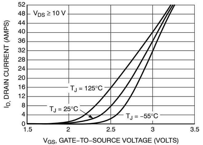
Figure 2. Transfer Characteristics
