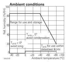
NOTE: For use conditions the temperature limits as indicated in the datasheets apply.
