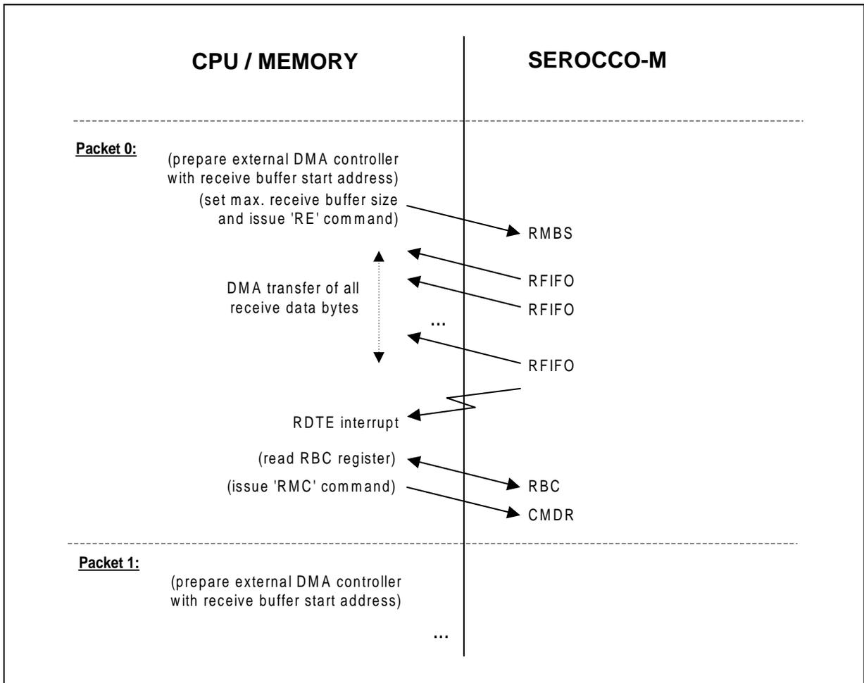
**Figure 60 DMA Receive (Single Buffer per Packet)**
