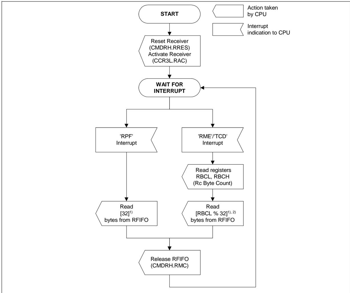
1) A receive threshold of 32 bytes is the default for HDLC/PPP mode. It can be programmed with bit field RFTH(1:0) in register CCR3H.
