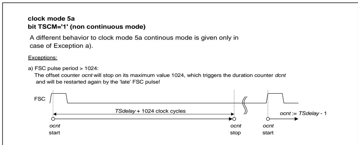
**Figure 23 Clock Mode 5a "Non Continuous Mode"**
