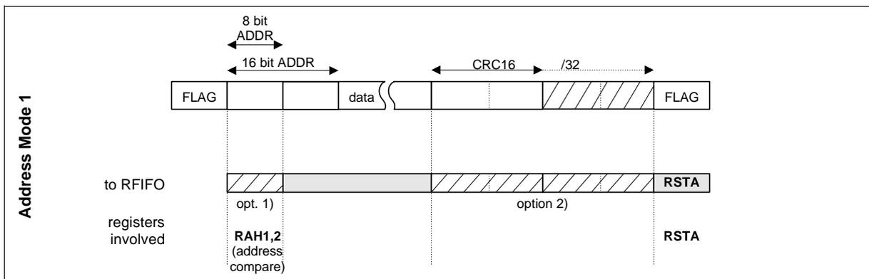
Figure 42 HDLC Receive Data Processing in Address Mode 1
