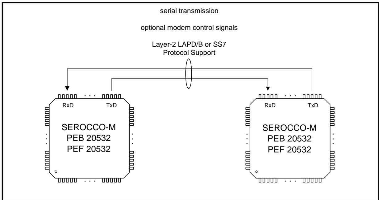
**Figure 4 Point-to-Point Configuration**
