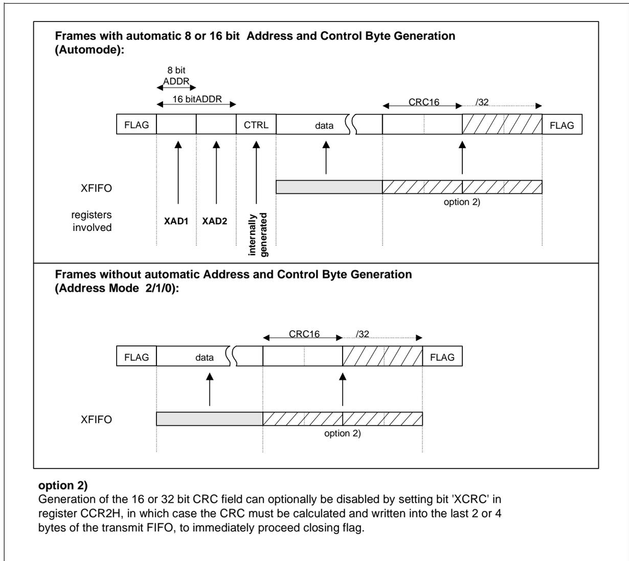
**Figure 44 SCC Transmit Data Flow (HDLC Modes)**
