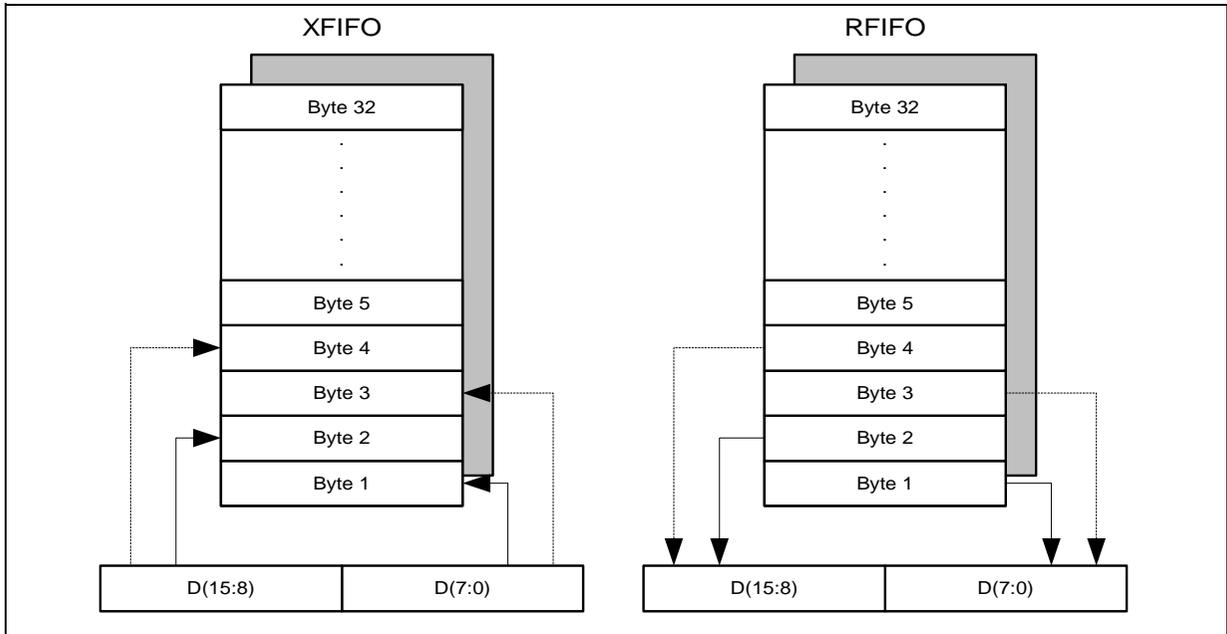
Figure 11 XFIFO/RFIFO Word Access (Intel Mode)
