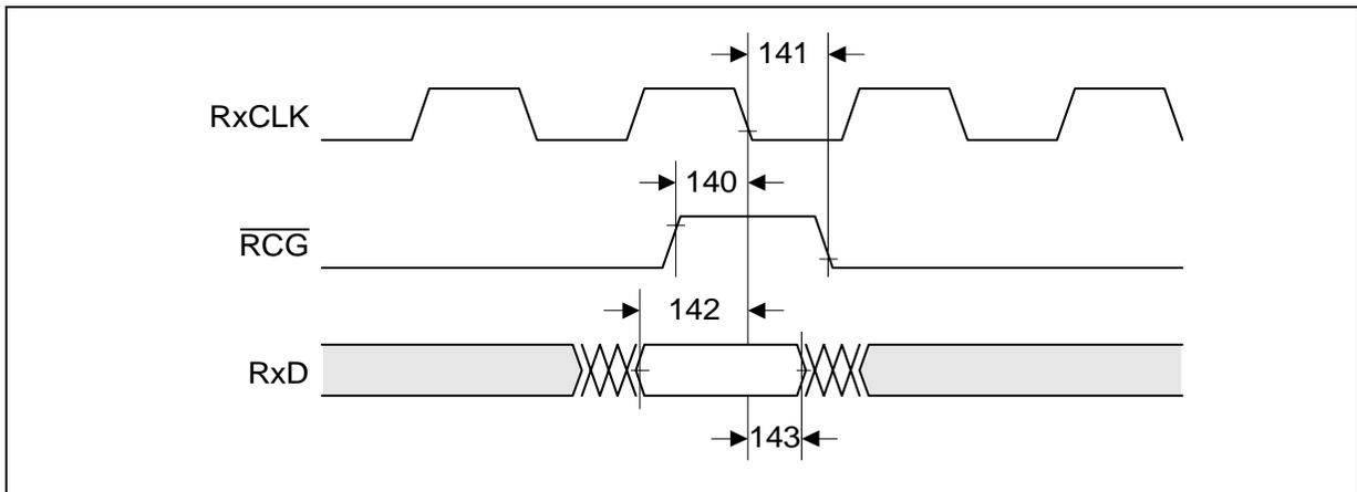
Figure 75 Clock Mode 4 Receive Gating Timing
