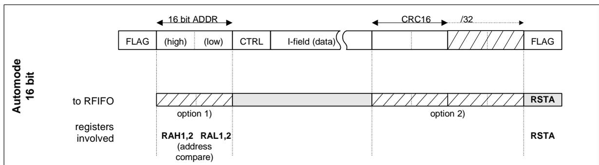
**Figure 38 HDLC Receive Data Processing in 16 bit Automode**
