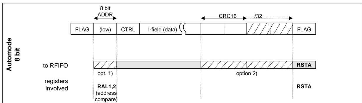
**Figure 39 HDLC Receive Data Processing in 8 bit Automode**
