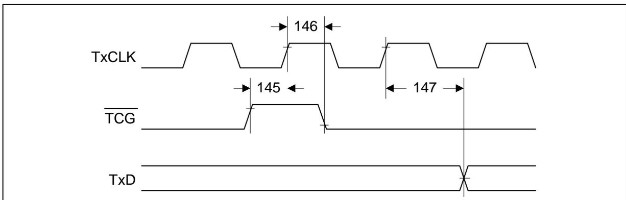
Figure 76 Clock Mode 4 Transmit Gating Timing
