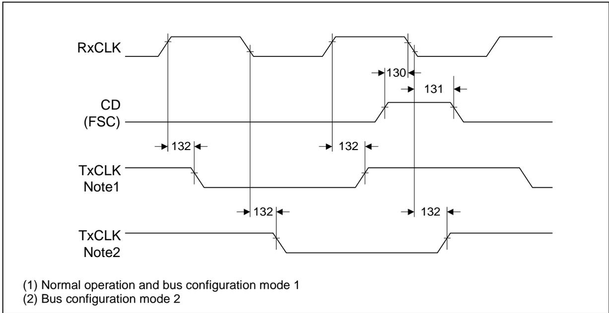
**Figure 77** Clock Mode 5 Frame Synchronisation Timing
