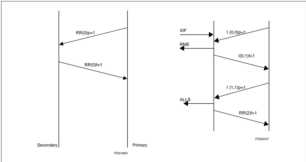
Figure 54 No Data to Send: Data Reception/Transmission
