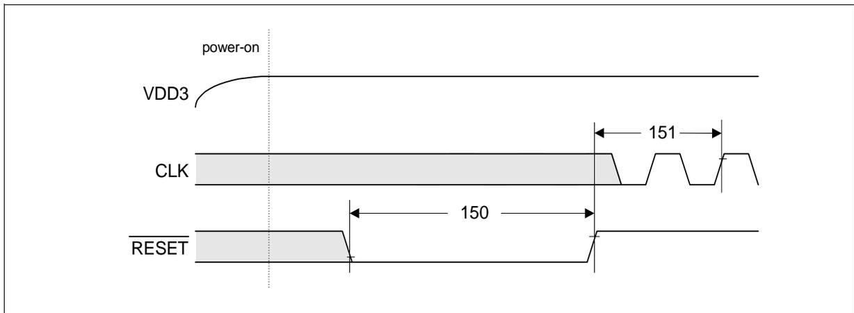
Figure 78 Reset Timing
