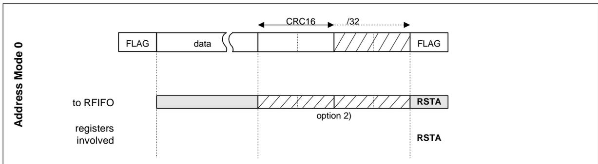
**Figure 43 HDLC Receive Data Processing in Address Mode 0**
