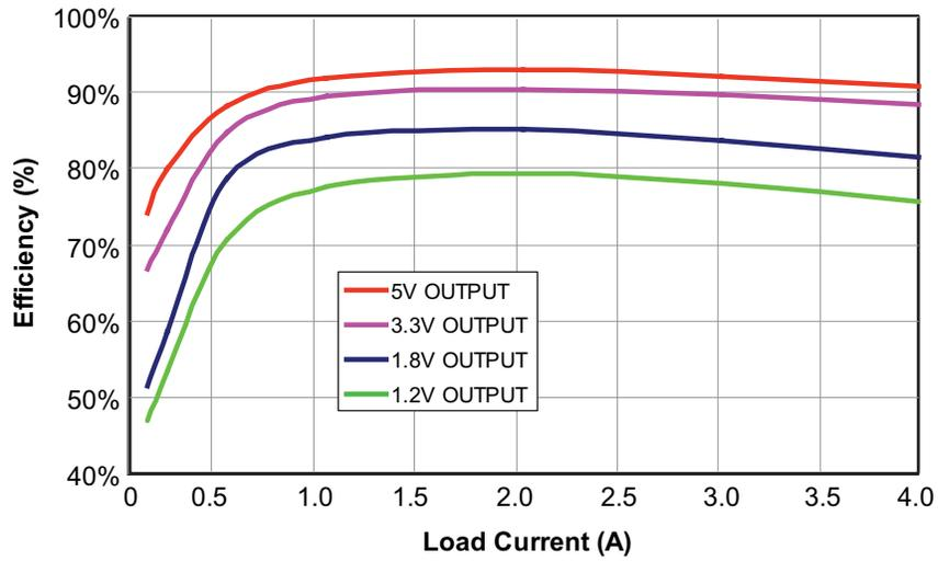
Efficiency ( $V_{IN} = 5V$ ) vs. Load Current
