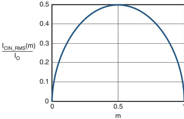
Figure 2. I<sub>CIN</sub> vs. Voltage Conversion Ratio
