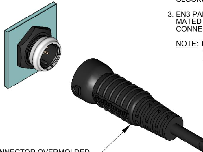
EN3 CORD CONNECTOR OVERMOLDED FOR QUICK CONNECT / DISCONNECT APPLICATIONS (PURCHASED SEPARATELY)
