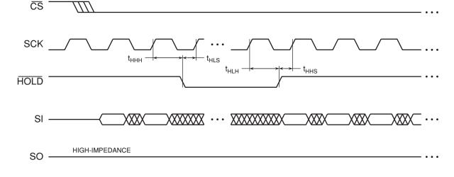
Figure 15-5.  $\overline{\text{HOLD}}$  Timing – Serial Output
