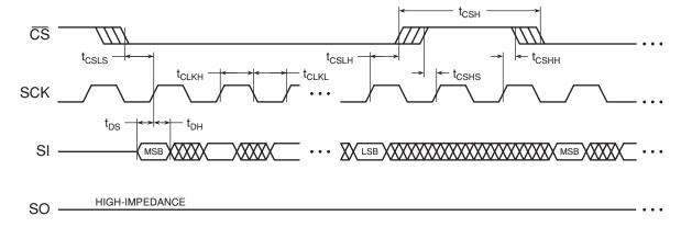
Figure 15-2. Serial Output Timing
