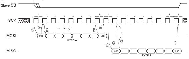
MOSI = Master Out, Slave In MISO = Master In, Slave Out The *Master* is the ASIC/MCU and the *Slave* is the memory device.
