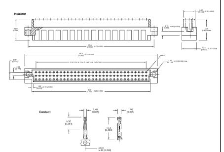
Elco's 3-row, 96 contact position receptacle connector with crimp contacts follows the pattern of the DIN 41612 standard. The innovative contact principle assures reliable electrical connection even under extreme conditions.
