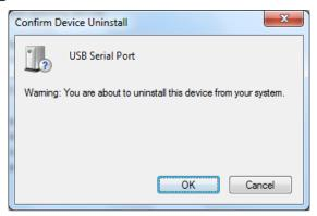
(9) Verify that the USB serial ports was deleted from the Device Manager.
