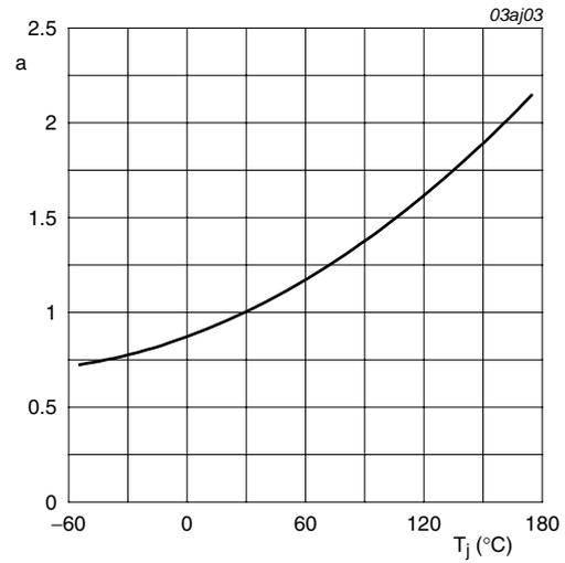
$$a = \frac{R_{DSon}}{R_{DSon(25^\circ C)}}$$
