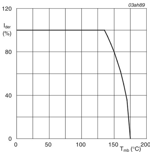
$$I_{der} = \frac{I_D}{I_{D(25^\circ\text{C})}} \times 100\%$$
