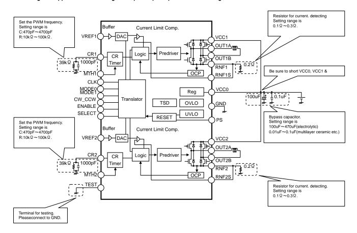
Fig.1 Block diagram & Application circuit diagram of BD6387EFV/BD6385EFV/BD6383EFV/BD6389FM
