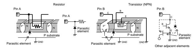
Fig. 4 Pattern Diagram of Parasitic Element
