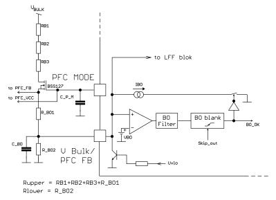
Figure 5. Internal Connection of the Brown-out Protection Block
