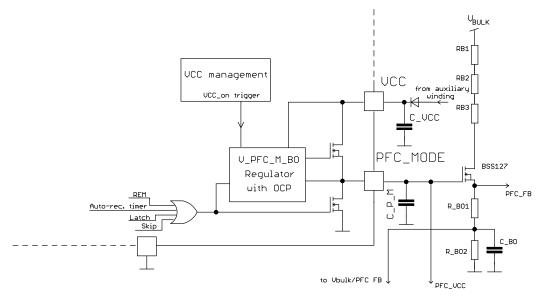
Figure 7. Internal Connection of the PFC MODE Block
