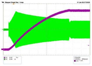
Figure 17. Application Startup with NCP13992 – Primary Current – Green, V<sub>out</sub> – Magenta
