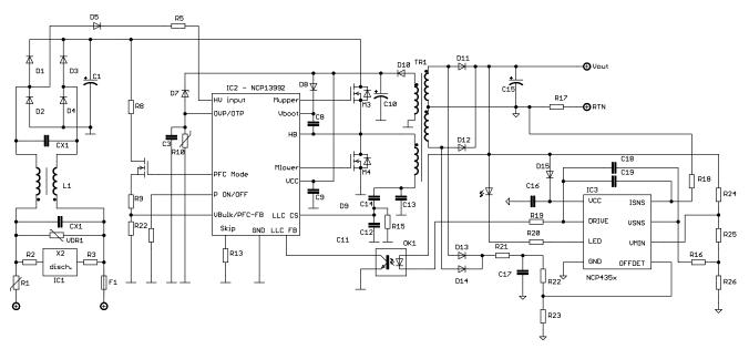
Figure 1. Typical Application Example without PFC Stage - WLLC Design
