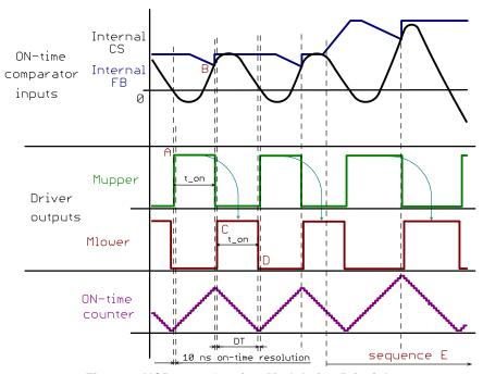
Figure 9. NCP13992 On-time Modulation Principle
