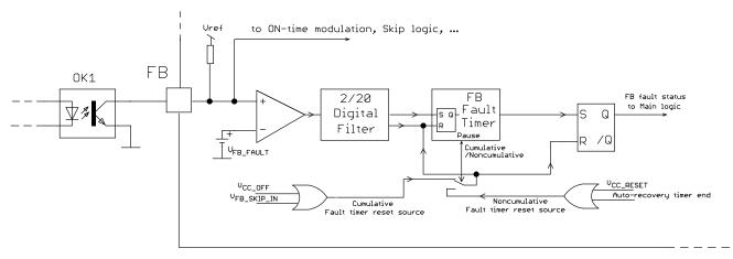
Figure 10. Internal FB Fault Management
