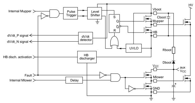
Figure 21. The NCP13992 Internal DRVs Structure
