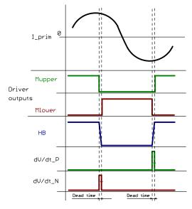
Figure 22. Optimum Dead-time Period Adjust
