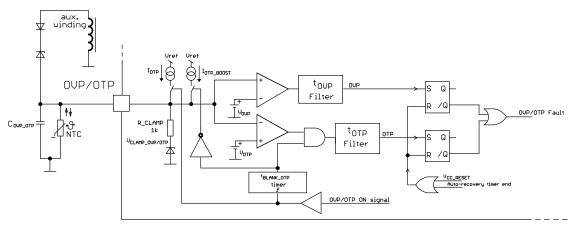
Figure 6. Internal Connection of OVP/OTP Input
