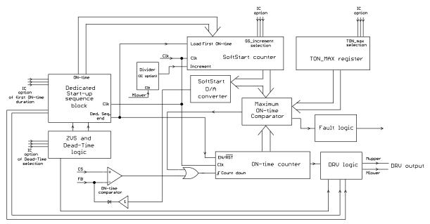
Figure 15. Soft-start Block Internal Implementation
