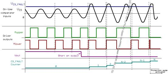
Figure 11. NCP13992 CS Fault Principle
