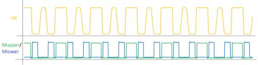
Figure 20. Light-load Operation
