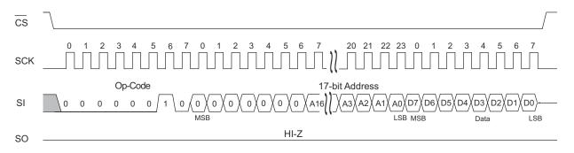
Figure 15. Burst Mode Write Instruction Timing
