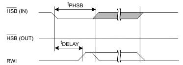
$\overline{\text{HSB}}$  pin is driven  $\underline{\text{HIGH}}$  to  $V_{CC}$  only by Internal 100 K $\Omega$  resistor,  $\overline{\text{HSB}}$  driver is disabled SRAM is disabled as long as HSB (IN) is driven LOW.
