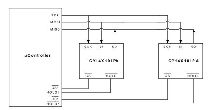
Figure 3. System Configuration Using SPI nvSRAM
