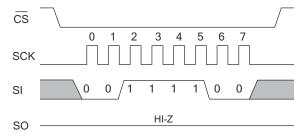
To issue this instruction, the device must be write enabled (WEN bit = '1'). The instruction is performed by transmitting the STORE opcode on the SI pin following the falling edge of CS. The WEN
