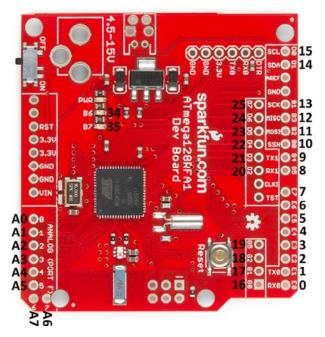
There are a few pins with **PWM functionality** – 3, 4, 5, 8, 9, 19, 34, and 35 – which you can use for analogWrite. Note that pins 34 and 35 are not broken out to pins. They're only connected to on-board LEDs.
