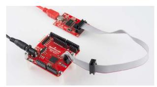
An AVR Pocket Programmer connected to the development board's ISP header. Straight headers were previously soldered to the header to allow for the connection.
