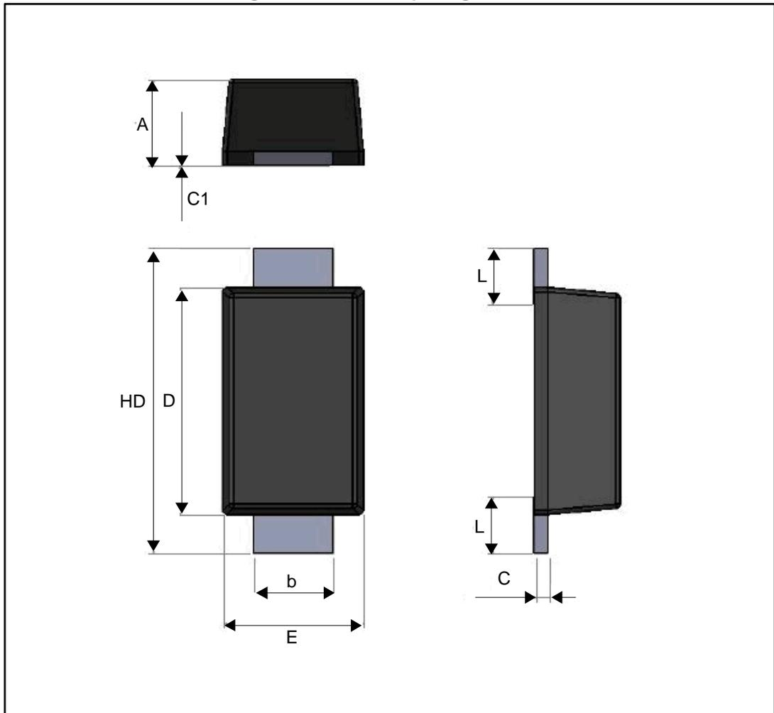
Table 5: SOD123Flat package mechanical data
