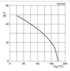
ig. 2. Normalized continuous drain current as a function of mounting base temperature
