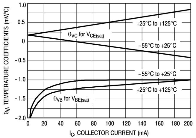
**Figure 12. Temperature Coefficients**
