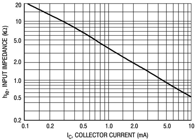
Figure 7. Input Impedance
