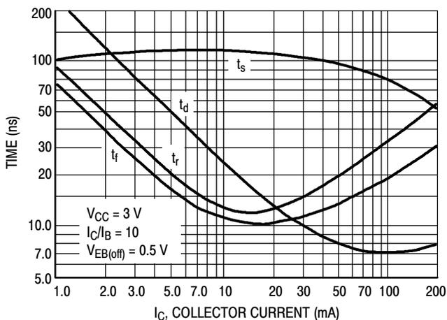
**Figure 2. Switching Times**
