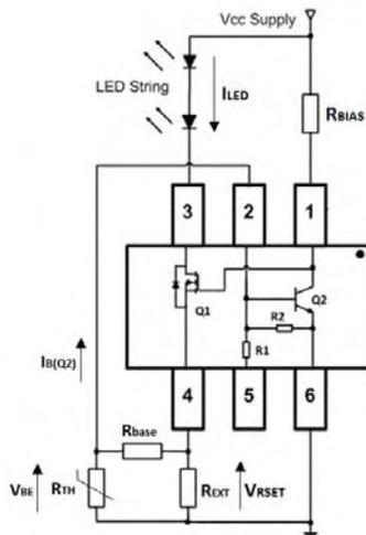
**Figure 14 Constant LED Current Temperature Compensation for AL5801**
