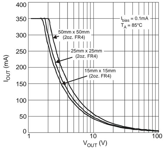
Figure 12 Output Current vs.  $V_{OUT}$
