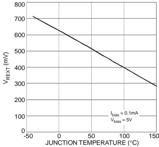
Figure 11  $V_{REXT}$  vs. Junction Temperature
