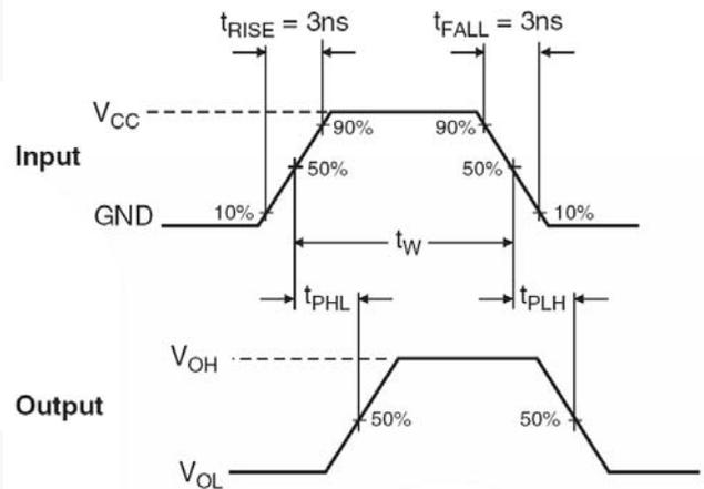
Figure 6. AC Waveforms for Inverting and Non-Inverting Functions
