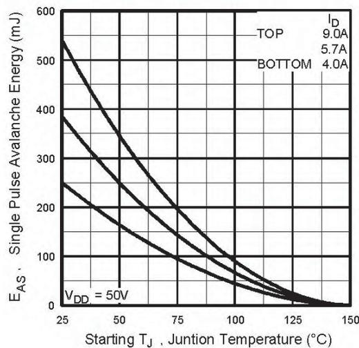
Fig. 12c - Maximum Avalanche Energy vs. Drain Current
