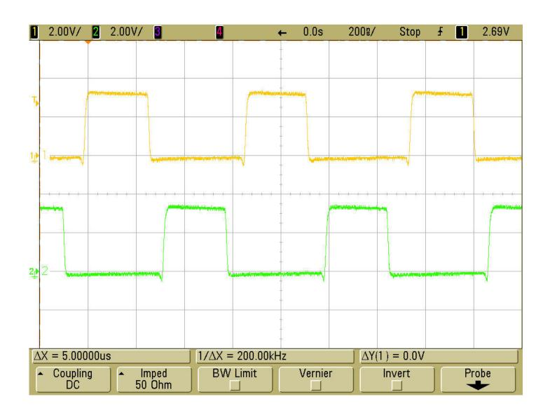
Figure 4. 180° Out-of-Phase Switching Operation  $V_{\text{IN}} = 3.3 \text{V}, \ V_{\text{OUT}} = 1.2 \text{V}, \ I_{\text{OUT}} = 5 \text{A}$
