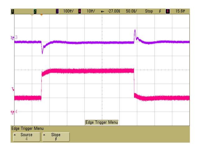
Figure 3. Load Step Response  $V_{IN} = 3.3V$ ,  $V_{OUT} = 1.8V$  & 10A Load Step Trace 1: Output Voltage (100mV/div AC) Trace 2: Output Current (5A/div)
