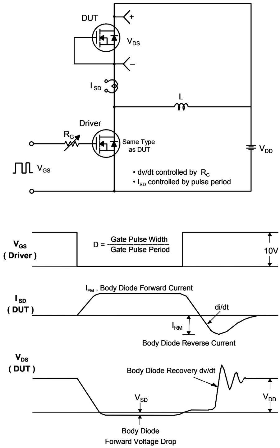
Figure 17. Peak Diode Recovery  $dv/dt$  Test Circuit & Waveforms
