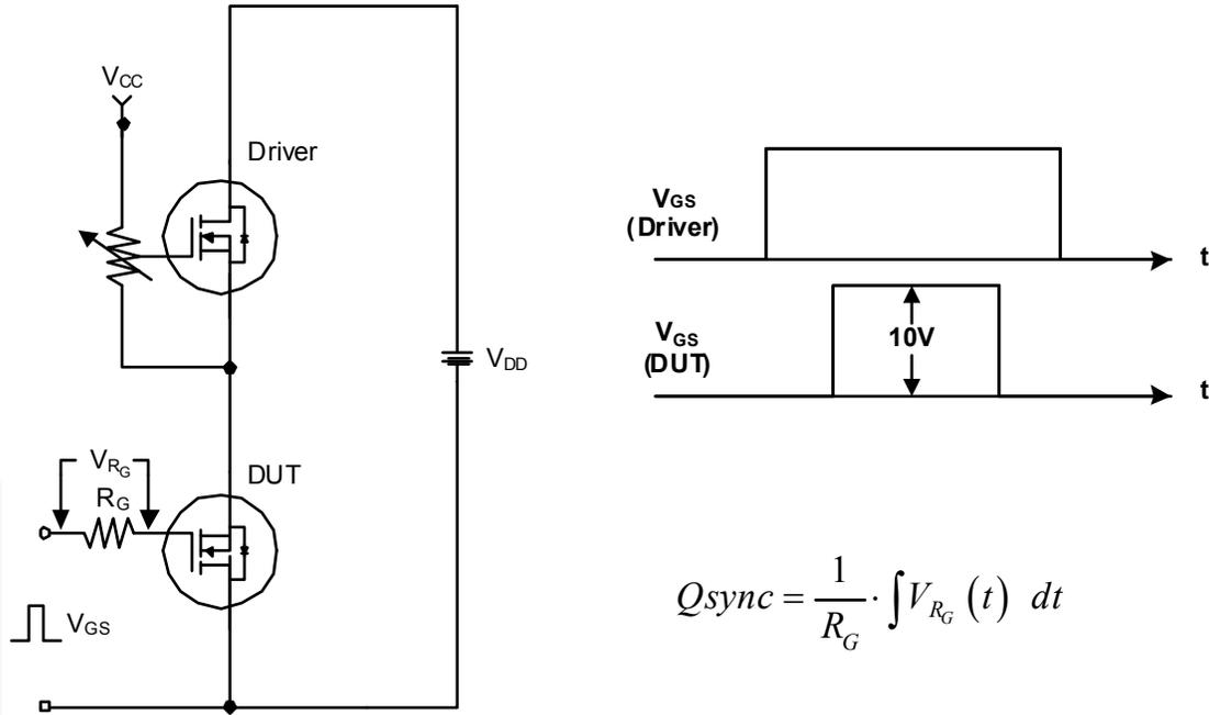
Figure 18. Total Gate Charge  $Q_{sync}$ . Test Circuit & Waveforms
