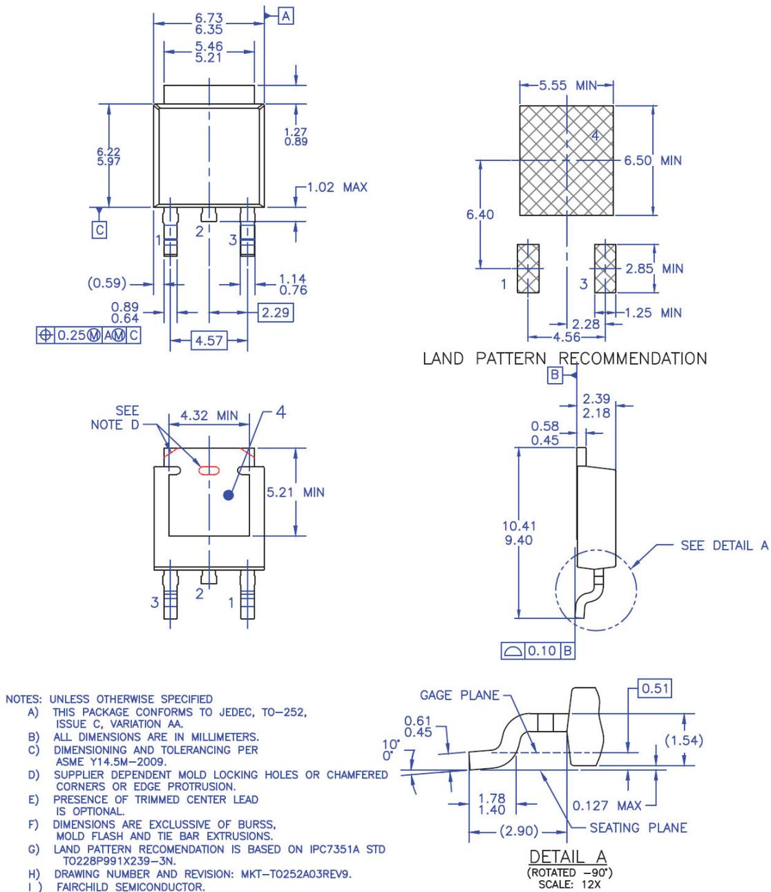
**Figure 19. TO252 (D-PAK), Molded, 3-Lead, Option AA&AB**
