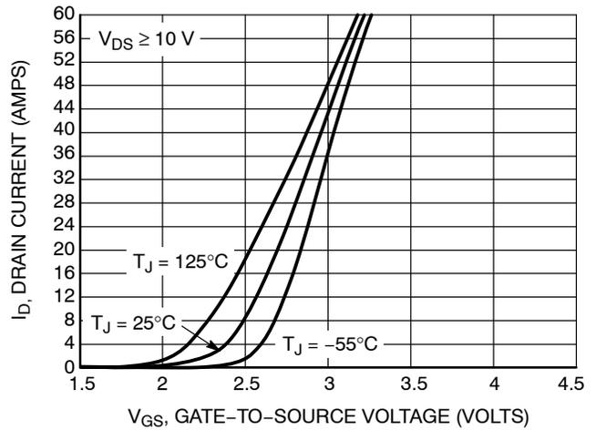
Figure 2. Transfer Characteristics
