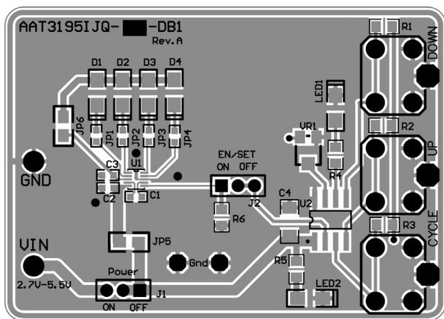
**Figure 4: AAT3195 Evaluation Board Top Side Layout.**
