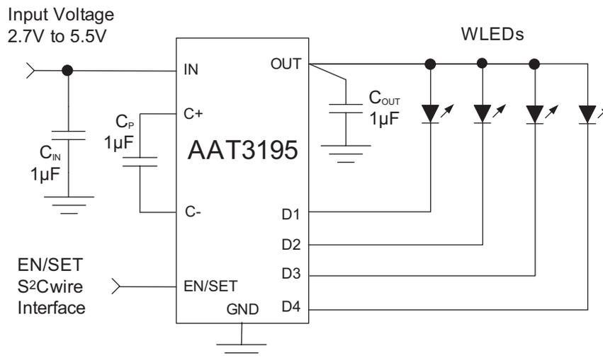
**AAT3195****Four-Channel Charge Pump LED Driver****Pin Descriptions**
