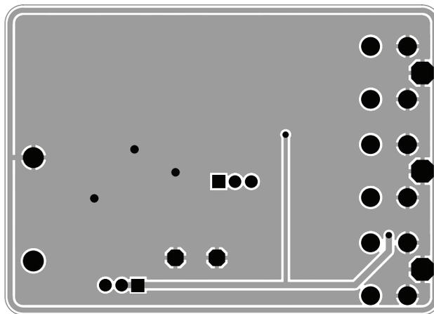
**Figure 5: AAT3195 Evaluation Board Bottom Side Layout.**
