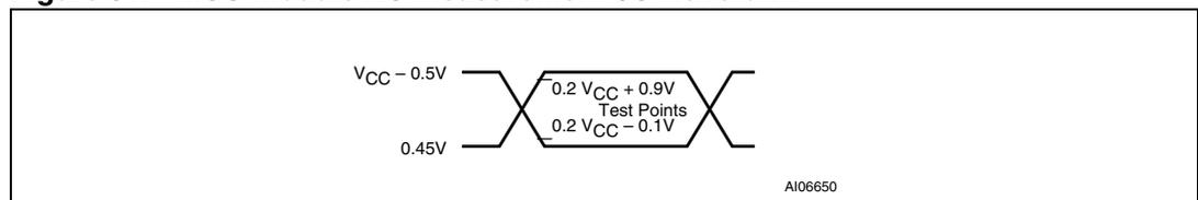
1. AC inputs during testing are driven at  $V_{CC}-0.5\text{ V}$  for a logic '1,' and  $0.45\text{ V}$  for a logic '0.'
