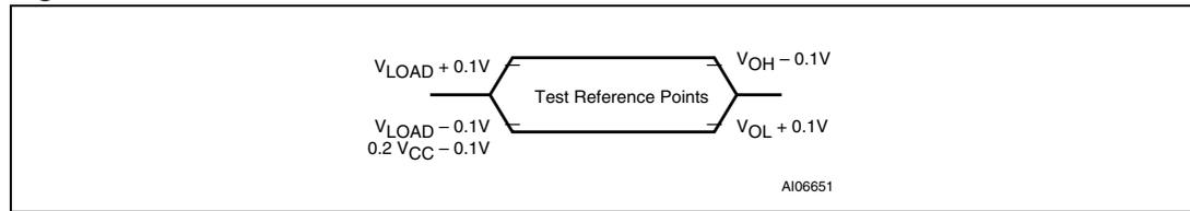
1. For timing purposes, a Port pin is considered to be no longer floating when a 100mV change from load voltage occurs, and begins to float when a 100mV change from the loaded  $V_{OH}$  or  $V_{OL}$  level occurs
