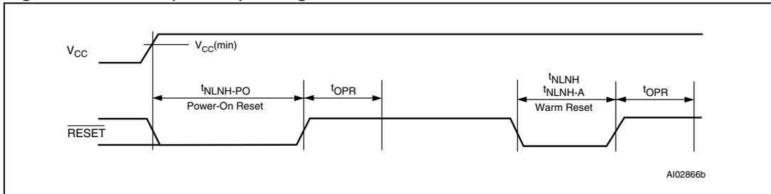
**Table 138. Reset ( $\overline{\text{RESET}}$ ) timing (5 V devices)**
