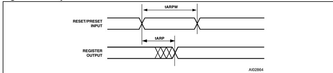
Figure 75. Asynchronous clock mode timing (product term clock)
