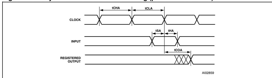
**Table 128. CPLD macrocell asynchronous clock mode timing (5 V devices)**
