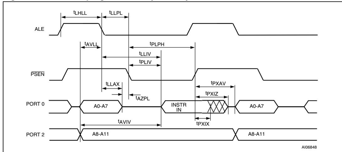
Table 117. External program memory AC characteristics (with the 5 V MCU module)
