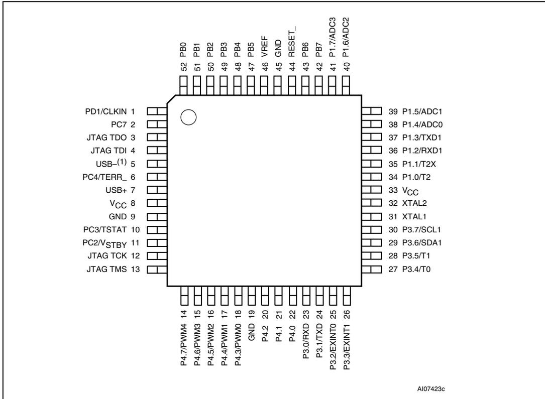
1. Pull-up resistor required on pin 5 (2 kΩ for 3 V devices, 7.5 kΩ for 5 V devices) for all 52-pin devices, with or without USB function.
