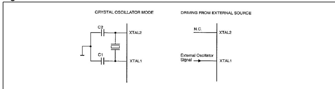
1.  $C1, C2 = 30 \text{ pF} \pm 10 \text{ pF}$  for crystals
