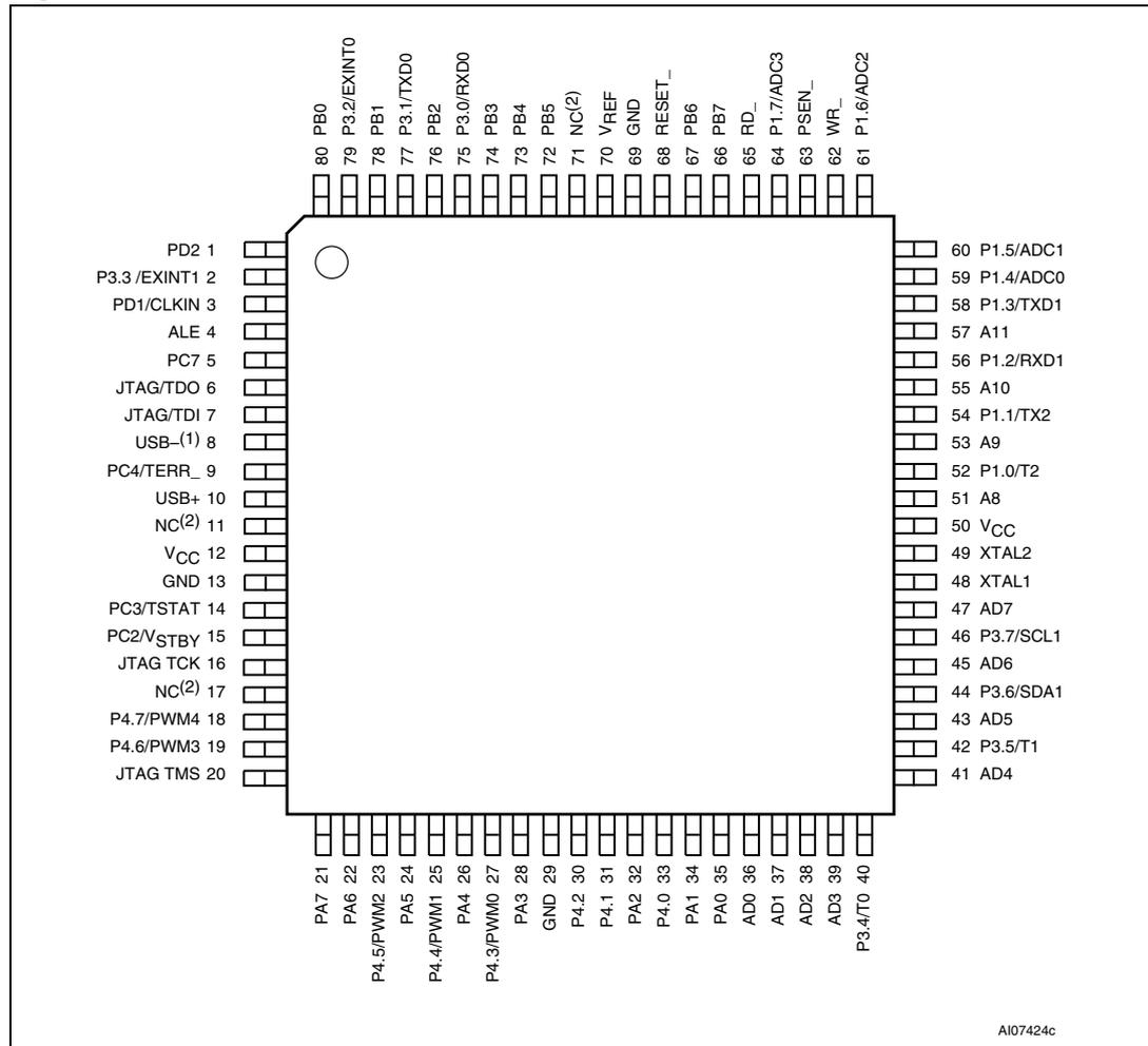
1. Pull-up resistor required on pin 8 (2 kΩ for 3 V devices, 7.5 kΩ for 5 V devices) for all 82-pin devices, with or without USB function.
