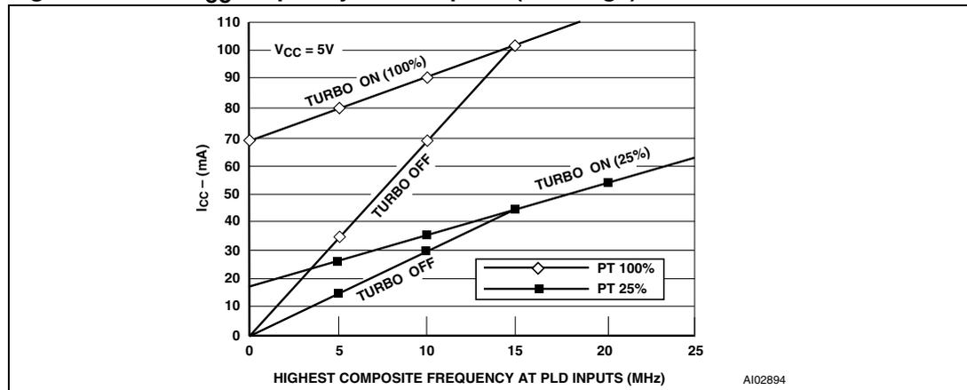
Figure 67. PLD  $I_{CC}$ /frequency consumption (3 V range)
