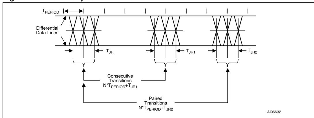
Figure 43. Differential to EOP transition skew and EOP width
