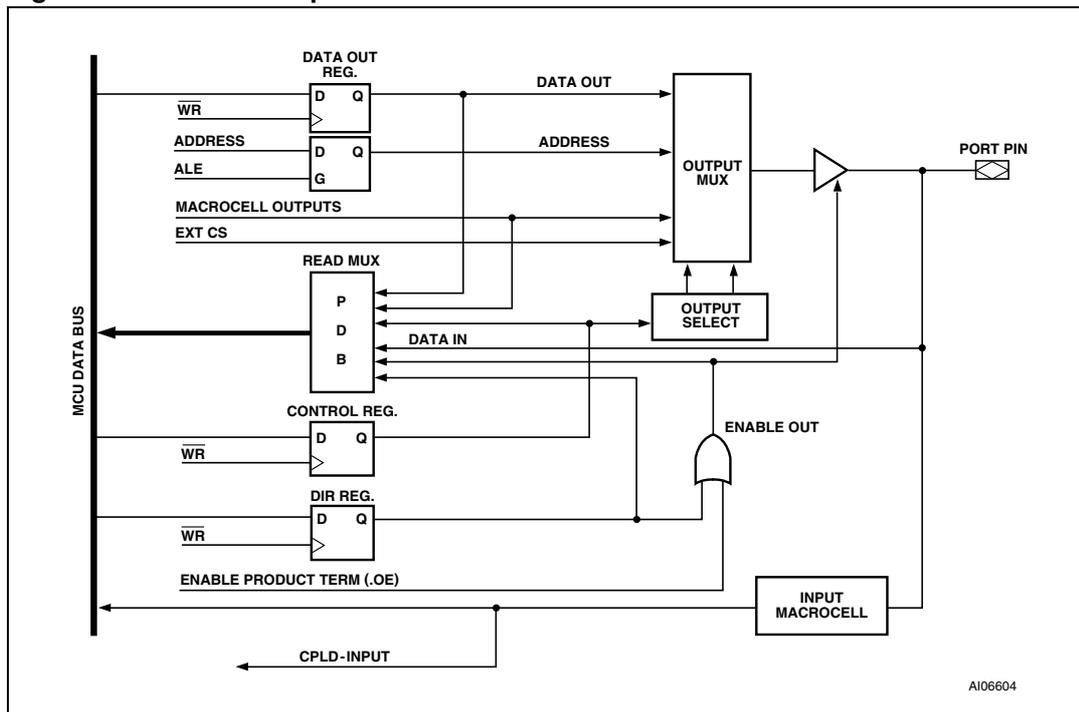
The Port pin's tri-state output driver enable is controlled by a two input OR gate whose inputs come from the CPLD AND Array enable product term and the Direction Register. If the enable product term of any of the Array outputs are not defined and that port pin is not defined as a CPLD output in the PSDsoft, then the Direction Register has sole control of the buffer that drives the port pin.
