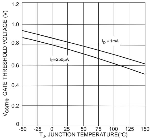
Fig. 7 Gate Threshold Variation vs. Ambient Temperature
