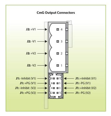
J1 CmG Signal Connector: Mating Connector J1: 8-way Molex: 87833-0831 Locking Molex: 51110-0860, Non-Locking Molex: 51110-0850; Locking and Polarizing: 51110-856 Crimp Terminal: Molex p/n 50394 Camden: CTB9350/4A Wurth Elektronik: 691 313 710 004 Camden: CTB9200/4A Wurth Elektronik: 691 352 710 004
