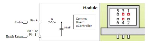
The CmB may be enabled/inhibited by means of a logic level signal applied to the enable input on Output Signal Connector J100x, Pin 4 (Positive), Pin 1 or 3 (Negative). The input voltage must be limited to no greater than 5 volts. When there is no connection, Pin 4 is HIGH (5V) and the module is enabled. Pulling Pin 4 to Common will disable the module.
