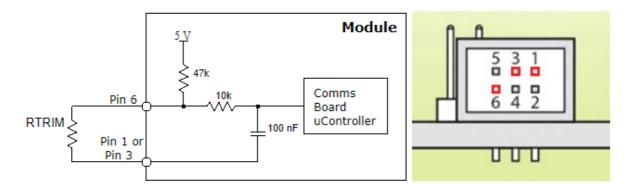
The output voltage of the CmA can be set by placing a resistor Rtrim across the Output Signal Connector J100x pins Vtrim (Pin 6) and Common (Pin 1 or Pin 3). The Rtrim resistance required for the users desired output voltage can be calculated using the following formula.
