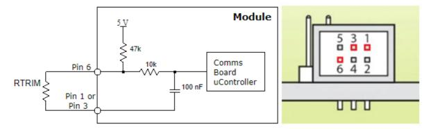
The output voltage of the CmC can be set by placing a resistor Rtrim across the Output Signal Connector pins Vtrim (Pin 6) and Common (Pin 1 or Pin 3). The Rtrim resistance required for the users desired output voltage can be calculated using the following formula.
