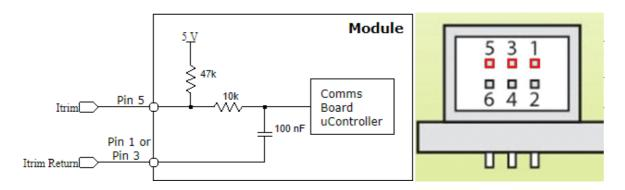
The current limit of the CoolMod can bet set by applying a control voltage Itrim across the Output Signal Connector J100x pins Itrim (Pin 5) and Common (Pin 1 or Pin 3). The Itrim voltage required for the users desired current limit with the CmA module can be calculated using the following formula.
