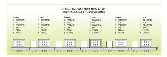
J1001-J1006 Mating Connectors J1001-J1006: 6-way Molex: 87833-0831 Locking Molex: 51110-0660; Non-Locking Molex 51110-0650; Locking and Polarizing Molex Crimp Terminal: Molex p/n 50394, or Molex 51110-0656 which includes Locking Tab & Polarization Keying,
