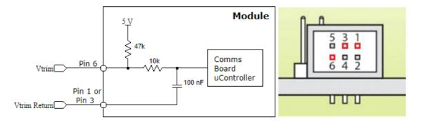
The output voltage of the CmE can be set by applying a control voltage Vtrim across the Output Signal Connector (J100x) pins Vtrim (Pin 6) and Common (Pin 1 or Pin 3). The Vtrim voltage required for the users desired output voltage can be calculated using the following formula.
