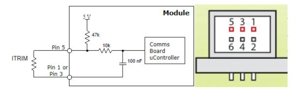
The current limit of the CoolMod can bet set by placing a resistor Rtrim across the Output Signal Connector (J100x) pins Vtrim (Pin 5) and Common (Pin 1 or Pin3). The Rtrim resistance required for the users desired output current limit can be calculated using the following formula along with the same table used to calculate Itrim.
