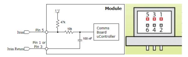
The current limit of the CoolMod can bet set by applying a control voltage Itrim across the Output Signal Connector (J100x) pins Itrim (Pin 5) and Common (Pin 1 or Pin 3). The Itrim voltage required for the users desired current limit with the CmD module can be calculated using the following formula.
