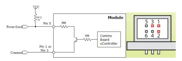
The CmA has a Power Good signal that is the output of an internal comparator which monitors the output voltage and determines whether this voltage is within normal operation limits. The Power
