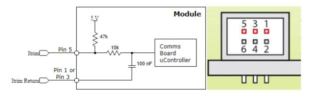
The current limit of the CoolMod can bet set by applying a control voltage Itrim across the Output Signal Connector (J100x) pins Itrim (Pin 5) and Common (Pin 1 or Pin 3). The Itrim voltage required for the users desired current limit with the CmC module can be calculated using the following formula.
