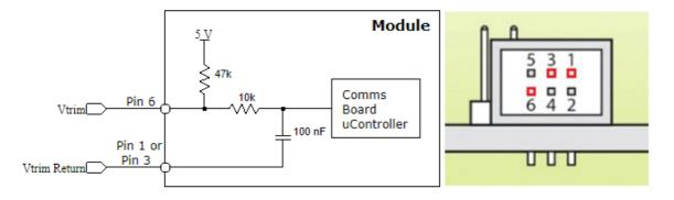
The output voltage of the CmD can be set by applying a control voltage Vtrim across the Output Signal Connector (J100x) pins Vtrim (Pin 6) and Common (Pin 1 or Pin 3). The Vtrim voltage required for the users desired output voltage can be calculated using the following formula.
