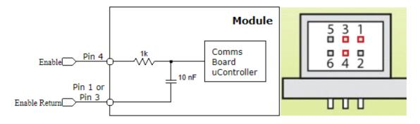
Both channels of the CmG may be enabled/inhibited by means of a logic level signal applied to the enable input on Output Signal Connector J100x, Pin 4 (Positive), Pin 1 or 3 (Negative). The input voltage must be limited to no greater than 5 volts. When there is no connection, Pin 4 is HIGH (5V) and the module is enabled. Pulling Pin 4 to Common will disable the module.
