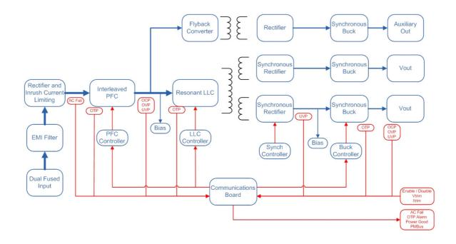
The CoolX platforms are comprised of an appropriate CoolPac and a selection of CoolMod DC output modules selected to deliver the exact volts and amps requirements of the system designer. An operational block diagram is shown above.
