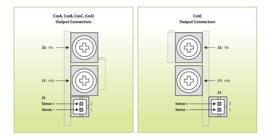
Remote sensing may be implemented by connecting the Positive Sense pin (J3 pin2) to the positive side of the remote load and the Negative Sense pin (J3 pin1) to the negative side of the remote load. The maximum line drop, which can be compensated for by remote sensing is 0.5V, subject to not exceeding the maximum module voltage at the output terminals. Observe the following precautions when remote sensing:
