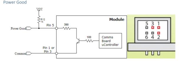
The CmD has a Power Good signal that is the output of an internal comparator which monitors the output voltage and determines whether this voltage is within normal operation limits. The Power
