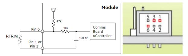
The output voltage of the CmE can be set by placing a resistor Rtrim across the Output Signal Connector pins Vtrim (Pin 6) and Common (Pin 1 or Pin 3). The Rtrim resistance required for the users desired output voltage can be calculated using the following formula.
