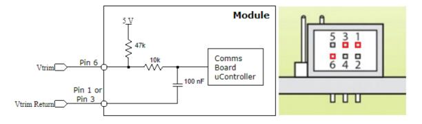
The output voltage of the CmB can be set by applying a control voltage Vtrim across the Output Signal Connector (J100x) pins Vtrim (Pin 6) and Common (Pin 1 or Pin 3). The Vtrim voltage required for the users desired output voltage can be calculated using the following formula.
