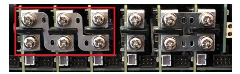
CmE Modules should not be connected in series. CmG outputs can be connected in series to each other, but there are no dedicated links for this, and should be done at a system level.
