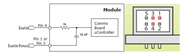
The CmE may be enabled/inhibited by means of a logic level signal applied to the enable input on Output Signal Connector J100x, Pin 4 (Positive), Pin 1 or 3 (Negative). The input voltage must be limited to no greater than 5 volts. When there is no connection, Pin 4 is HIGH (5V) and the module is enabled. Pulling Pin 4 to Common will disable the module.
