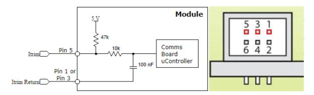
The current limit of the CoolMod can bet set by applying a control voltage Itrim across the Output Signal Connector (J100x) pins Itrim (Pin 5) and Common (Pin 1 or Pin 3). The Itrim voltage required for the users desired current limit with the CmB module can be calculated using the following formula.
