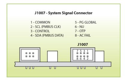
J1007 System Signal Connector Mating Connector J1007: 8-way Molex: 87833-0831 Locking Molex: 51110-0860, Non-Locking Molex: 51110-0850; Locking and Polarizing Molex: 51110-0856 Crimp Terminal: Molex p/n 50394
