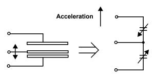
Figure 3. Transducer Physical Model
