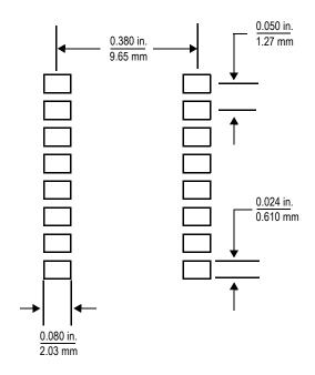
Figure 7. Footprint SOIC-16 (Case 475-01)
