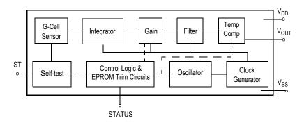
Figure 3. Simplified Accelerometer Functional Block Diagram
