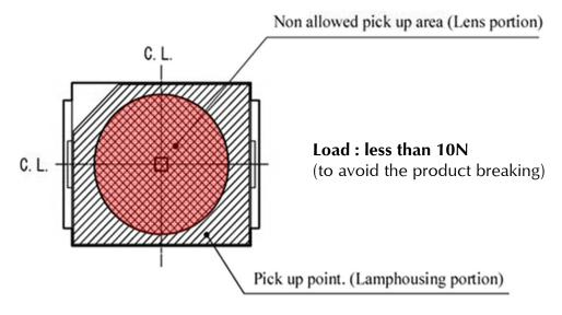
Please adjust the load, the pick up point, the nozzle diameter, etc. before mounting because the over load can cause the breakage of the lamp housing.
