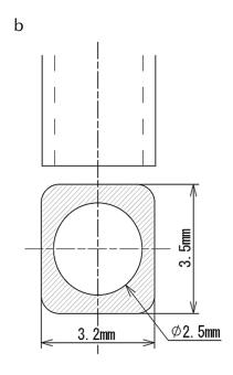
Nozzle with chamfering is recommended
